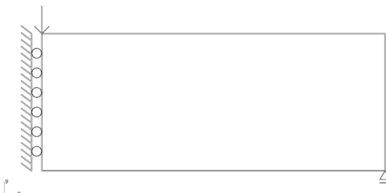
Figure 6.1: Half MBB beam used to compare the results of changing parameters
