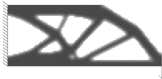
Figure 6.11: Optimised result without considering additive manufacturing constraints
