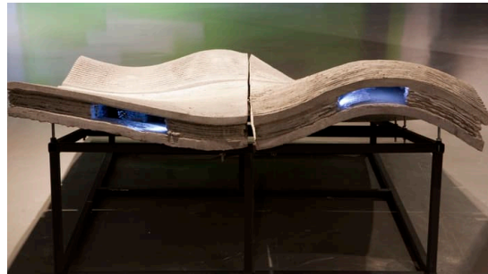
Figure 2.6: Concrete Printing at Loughborough University (lboro.ac.uk 2011)
