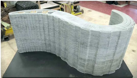
Figure 2.6: Concrete Printing at Loughborough University (lboro.ac.uk 2011)
