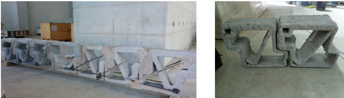
Figure 2.11: 3D printed modulated concrete beam (wasproject.it 2015)
