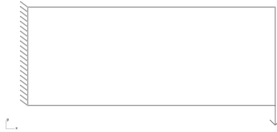
Figure 6.10: Cantilever problem used to compare the results of changing parameters
