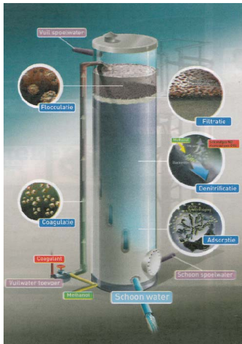
Figure 7.3: 1-Step filter for removal of nitrate, phosphate and organic micropollutants (van de Sandt, 2009)
