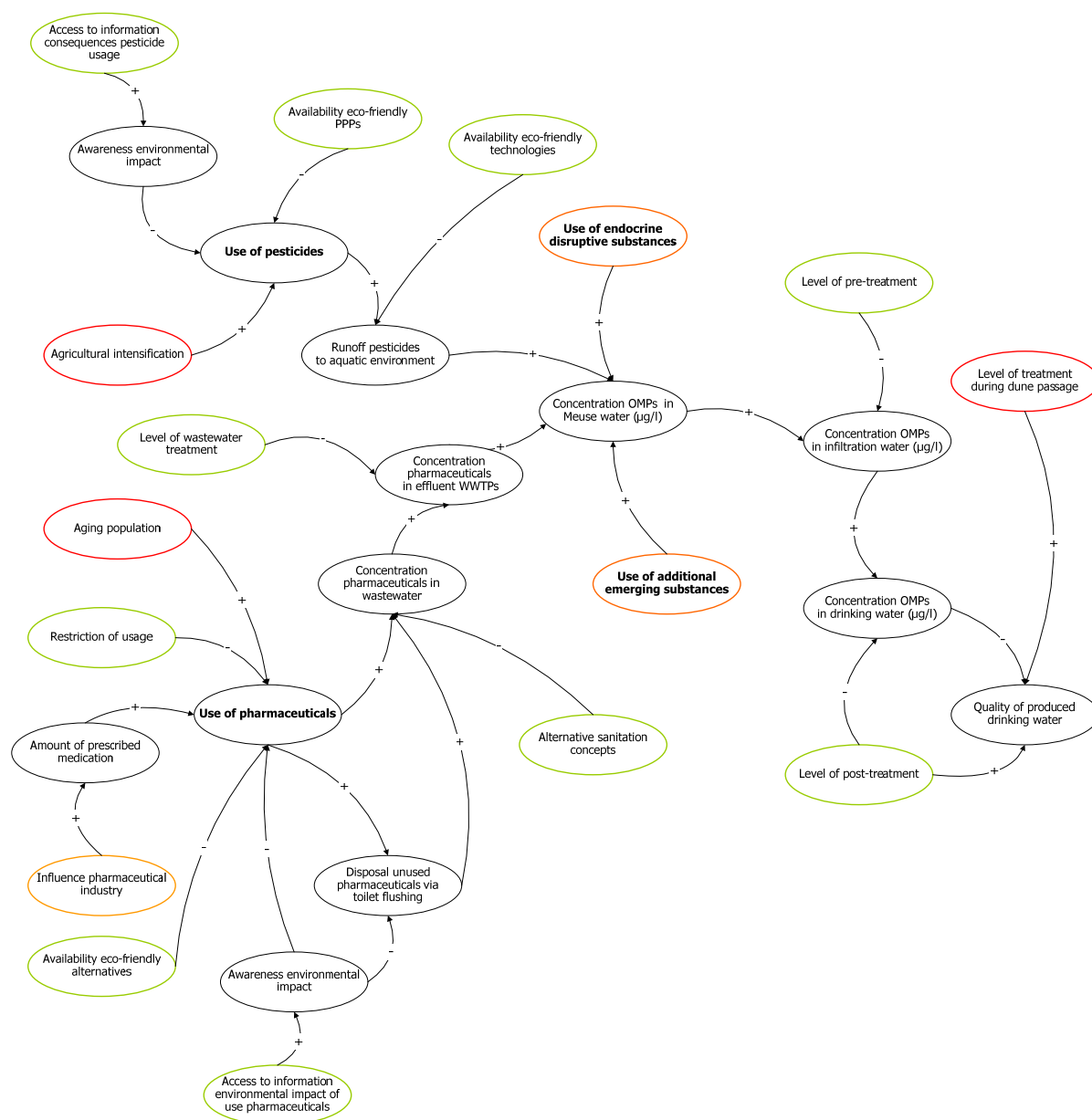
Figure A2.1: Cause and effect diagram
