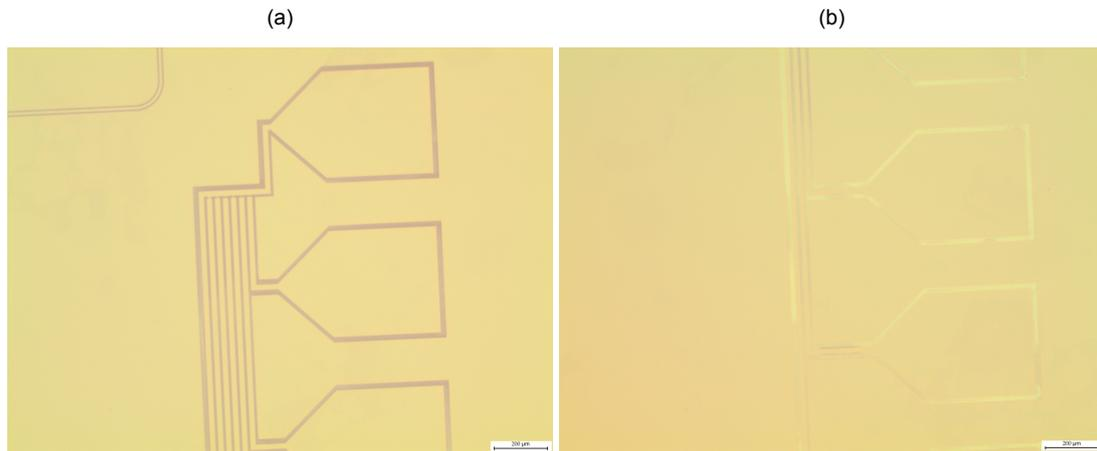
Figure 3.9: a) One end of the sample is etched successfully. Shown is part of an array of contact pads, the top of which serves as a common ground for the rest. b) The other end of the same array of contact pads (and connections between them) is under-etched, there is still MoRe covering the Si where it should have been removed.
