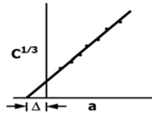
Figure 6. \Delta is a factor for the modified beam theory (standard test method ASTM D5528).
