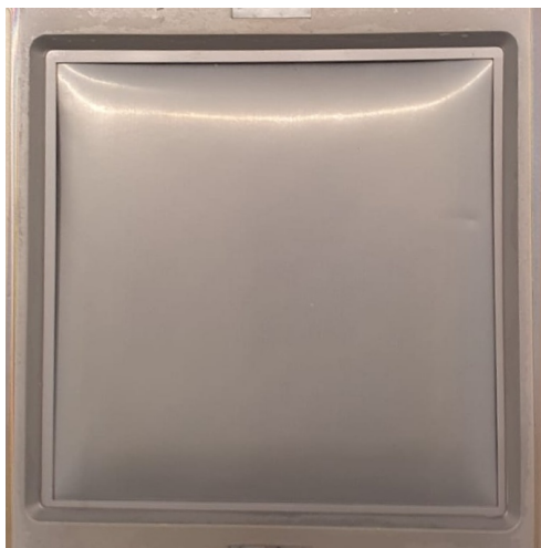
Figure 3.12: Appearance of Silicon deposited on the aluminium using AMIGO.
