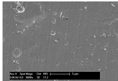
Figure 3.7: Baseline texturing of Aluminium + FTO used in industry. Figure 3.8: Baseline texturing of Aluminium used in industry. SEM Generated by GenPro4, AFM data measured by D.Rajagopal[49] image by D.Rajagopal[49].
