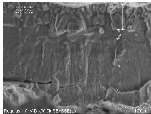
Figure 3.30: Measured thickness of tandem cell after all processes. The resolution is low due to low electron acceleration.
