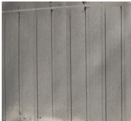
Figure 3.13: Appearance of cells after scribing. The thin lines are laser scribe and dark lines are lift off ink.
