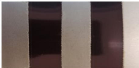
Figure 3.14: The cell after substrate etching. Area of solar cell: 2.5\text{cm}^2 . The protected area in the etching forms bus bar.
