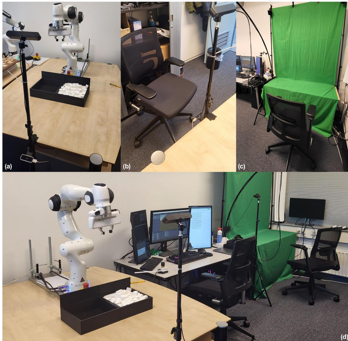
FIGURE 2 (a) Franka Emika Panda robot arm featuring the box-and-block task in front. The tripod holding the ZED2 stereo camera and the Leap sensor directed towards the seated participant from below is also visible. (b) Seating location for the participant when controlling the robot in the real environment. (c) Green screen setup with seating position for the participant when controlling the robot in the teleoperation conditions. The Varjo XR-3, connected to a cable boom, is visible on the left side, and two SteamVR base stations are positioned at the top corners of the green screen. (d) Photograph of the entire setup, depicting the experimenter's computer positioned between the robot arm and the green screen.
