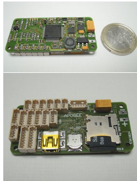
Figure 10: Apogee autopilot controller board
