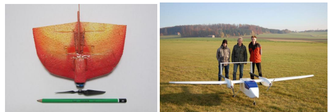
Figure 2: Quark and Adler UAV as two examples of Paparazzi flying fixed-wing aircrafts
