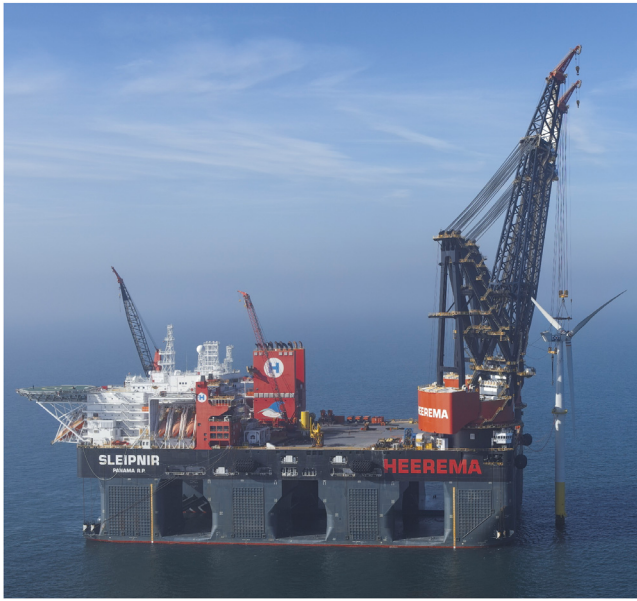
Fig. 1. Semi-submersible crane vessel Sleipnir of Heerema Marine Contractors performing a floating offshore installation of an OWT (DOB-Academy, 2022).
