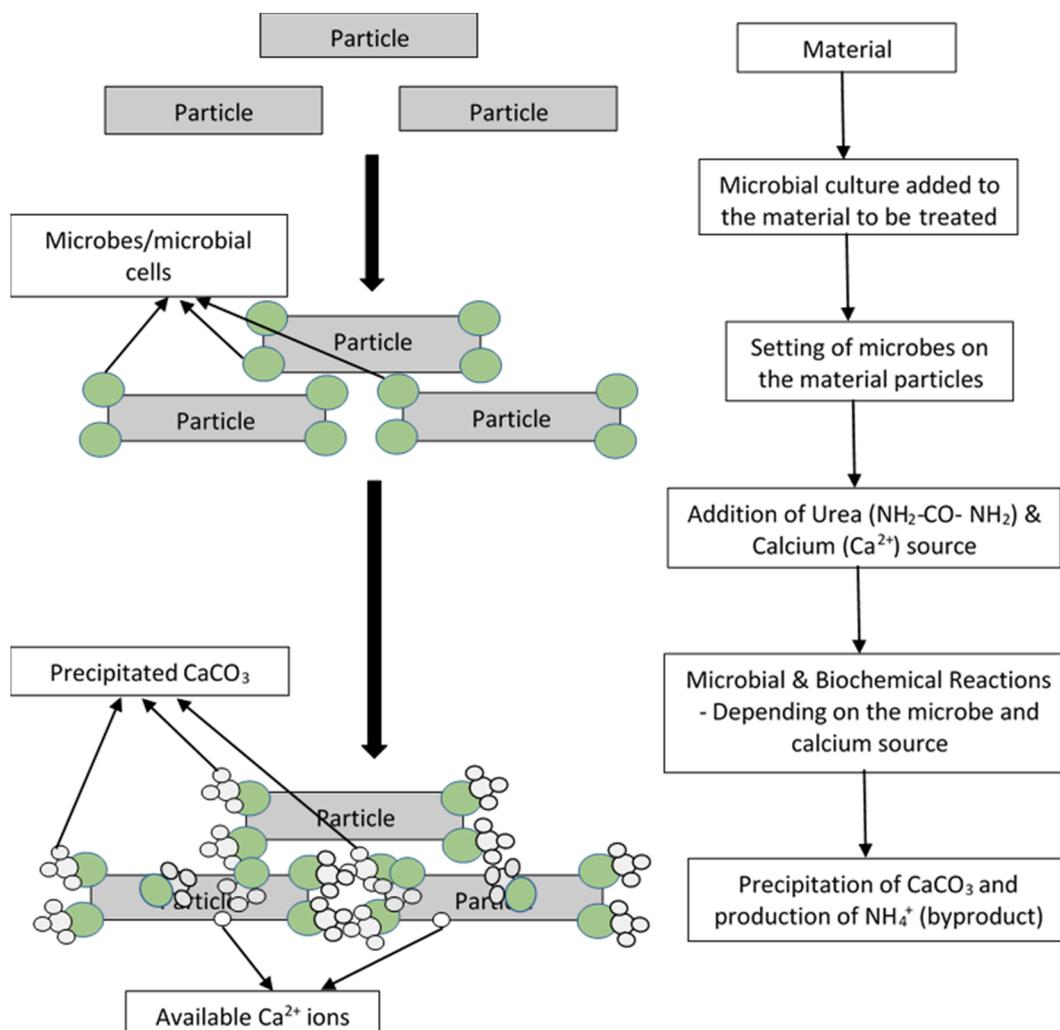
Fig. 2. Typical mechanism of MICP/EICP via urea hydrolysis.
