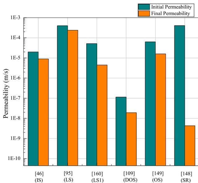
Fig. 6. Reduction in permeability before and after the treatment IS - Iiterbeck sand, LS - Loose sand, LS1 - Lateritic soil, DOS - Dry Ottawa sand, OS - Organic soil, SR - Sand with radioactive effluent.
