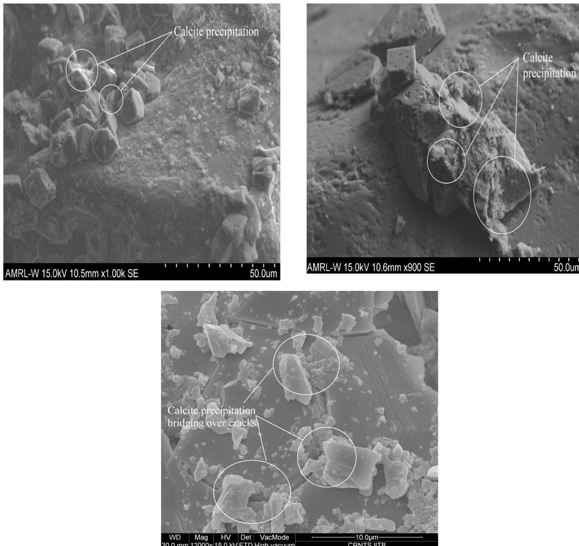
Fig. 7. Typical SEM images depicting microbially induced calcite precipitation (Images Courtesy: AMRL, University of Strathclyde and CRNTS, IIT Bombay).
