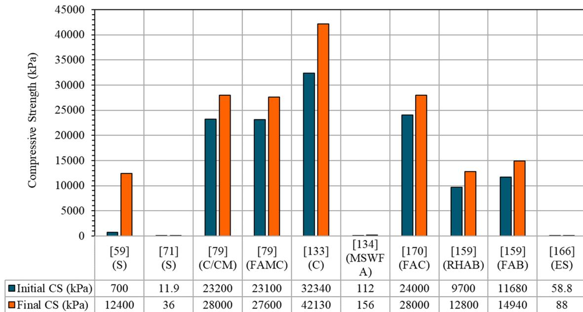
Fig. 4. Improvement in compressive strength (CS) after MICP/EICP treatment Where, S- Sand, C- Concrete, CM- Cement Mortar, FAMC- Fly Ash- amended Mortar & Concrete, FAC- Fly Ash Concrete, RHAB- Rice Husk Ash Bricks, FAB- Fly Ash Bricks, ES- Expansive Soil, MSWFA- Municipal Solid Waste Fly Ash.
