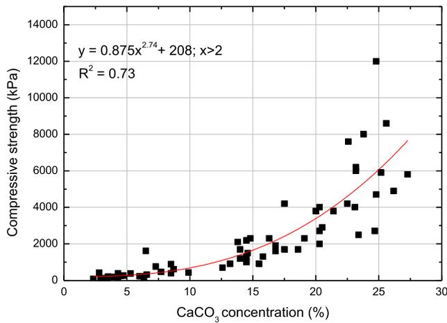
Fig. 5. Compressive strength versus CaCO<sub>3</sub> concentration.
