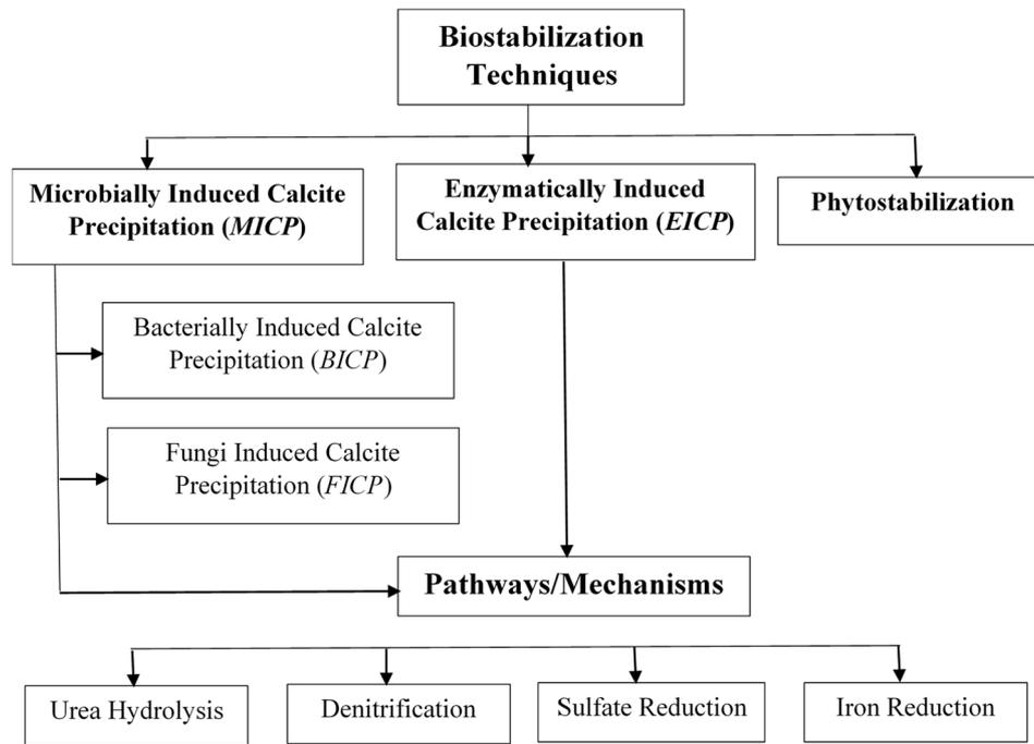
Fig. 1. Biostabilization techniques and their mechanisms.
