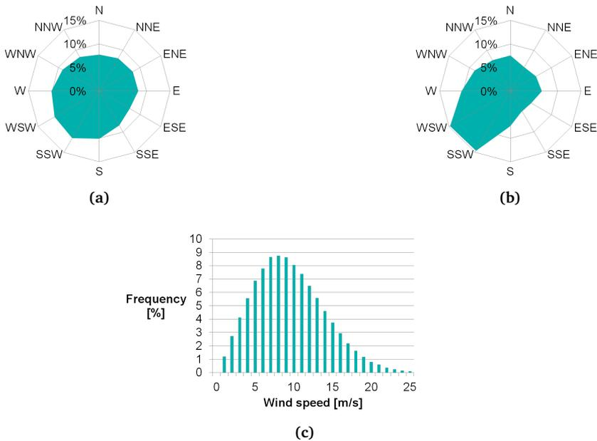
**Figure D.1:** Wind climate of Hollandse Kust Zuid. Expressed are the mean wind speed (a) and frequency (b) distribution with respect to the wind direction and the frequency distribution of wind speed (c).
