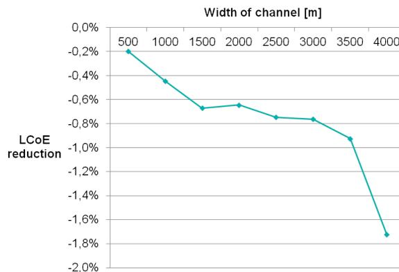
Figure 6.11: Reduction in LCoE against variation of the glacial channel width.
