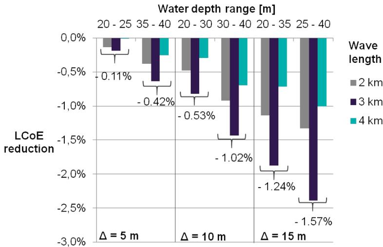
**Figure 6.22:** LCoE reduction for different variations of sand dunes. Variations include wave length indicated with the legend and water depth range indicated at the x-axis. The peak-to-trough range is indicated with  $\Delta$ . Furthermore, for every particular water depth range the average LCoE reduction is indicated.
