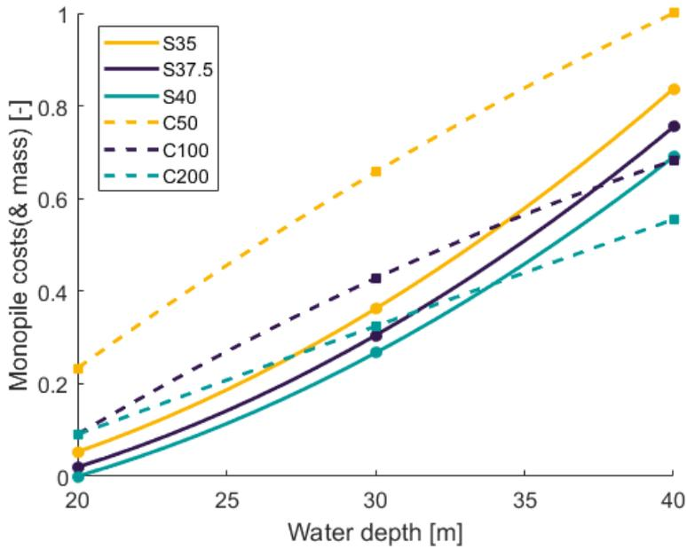
**Figure 5.2:** MP costs (& mass) against the water depth for variations in uniform soil types. The estimations are normalized for confidentiality reasons between 0 and 1, with 0 not reflecting an absolute zero in real values. The indicators display the points for which designs are created. The plotted line is based on spline interpolation.
