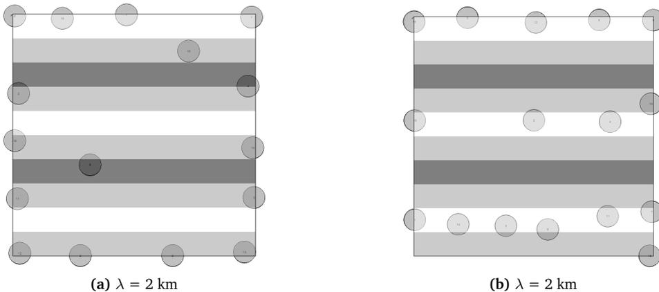
**Figure 6.23:** Wind-turbine layouts with original (left) and improved (right) OWFLO for a water depth range of 20 - 35 m, and varying wave lengths.
