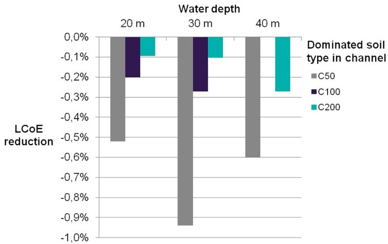
**Figure 6.8:** LCoE reduction against variations in clay soil type inside the channel at different water depths.
