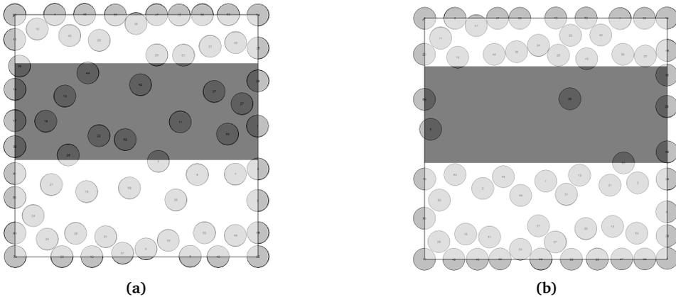
**Figure 6.21:** Dense OWF containing 64 WTs having a glacial channel width of 2000 m. Wind-turbine layouts are created with original (a) and improved (b) OWFLO.
