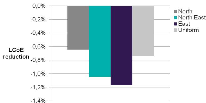
**Figure 6.15:** LCoE reduction against dominant wind direction.
