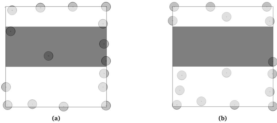
**Figure 6.18:** Wind-turbine layout for E dominated wind direction. Layouts are created with original (a) and improved (b) OWFLO.
