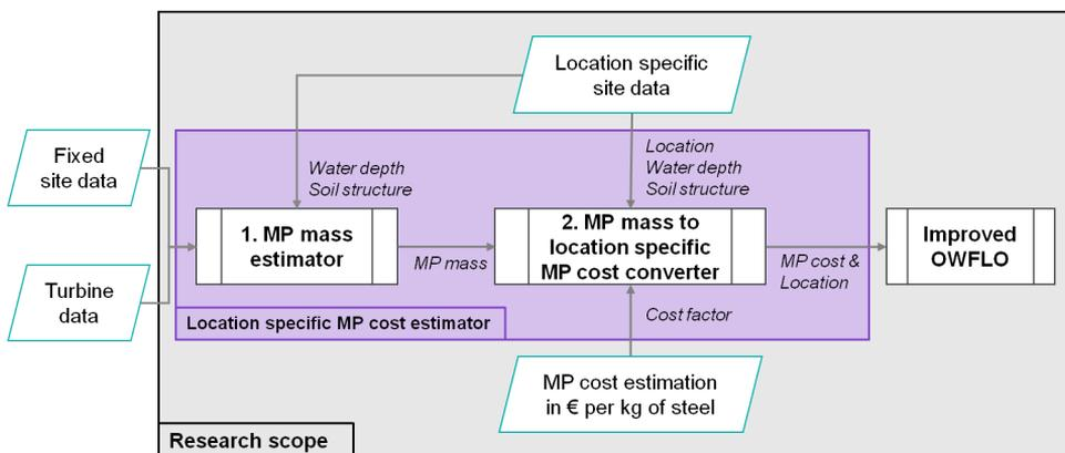
**Figure 4.4:** Process-flow diagram of the method incorporated in a model able to estimate MP costs at specific locations within an OWF.
