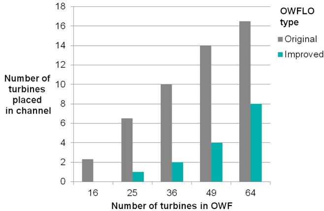
**Figure 6.20:** Number of WTs placed in the glacial channel for original and improved OWFLO against the number of wind turbines placed inside the OWF.
