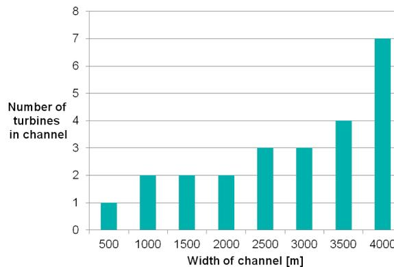
Figure 6.12: Number of WTs placed in channel with original OWFLO.
