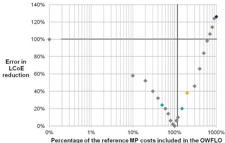
**Figure 3.4:** Results of the sensitivity study. On the x-axis the percentage of the reference MP costs included in the OWFLOs, this expresses the error in MP cost estimation. The y-axis expresses the resulting deviation in LCoE reduction.
