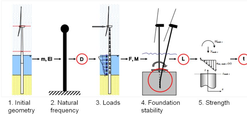
**Figure 4.1:** Visualisation of the design steps. Indicated is at which steps the adjustments of the diameter, length and wall thickness take place [68].
