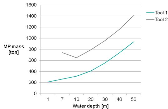
**Figure C.1:** MP mass estimations with Tool 1 & 2. Designs based on sand dominated soil with a friction angle of  $37.5^\circ$ . Visualising the shortcoming of Tool 2 to make proper designs at water depths below 10 m.
