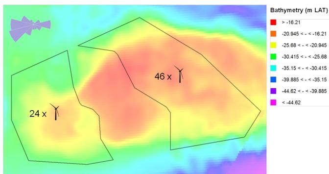
**Figure 6.7:** Impression of the Krieger's Flak offshore wind farm. Indicated are the site boundaries, bathymetry, and the frequency distribution of the wind direction.
