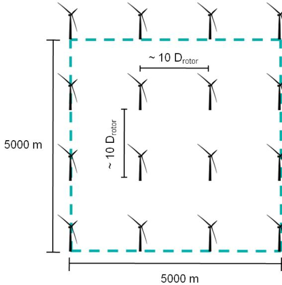
**Figure 2.2:** Dimensions of the hypothetical OWF. The 16 WTs are symmetrically distributed in a square with  $\sim 10D_{rotor}$  spacing, resulting in a 5000 x 5000 m site.
