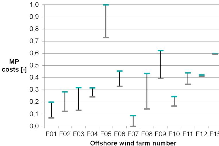
**Figure 3.1:** MP-cost variation of MP designs within several OWFs. Indicated are the upper and lower boundaries of MP costs within the OWFs. For confidentiality reasons the costs are normalized between 0 and 1, with 0 being the lowest MP cost available.
