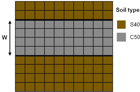
**Figure 6.3:** Visual expression of how a glacial channel having a width (W) of 2000 m is simulated.
