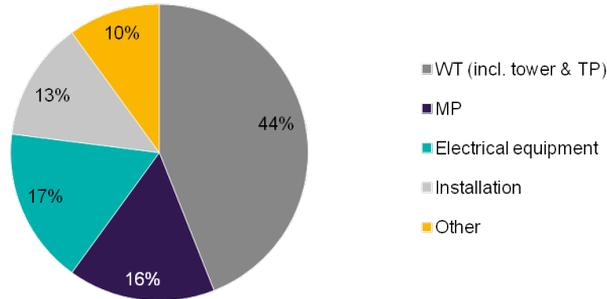
**Figure 2.3:** CapEx breakdown of an OWF project [17]. This CapEx breakdown is used to estimate the electrical equipment, installation and other costs based on the values of the WT and MP costs, and the percentage of their share in the breakdown.
