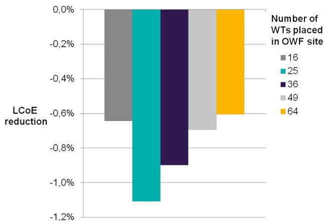
**Figure 6.19:** Reduction in LCoE against the number of WTs placed within the OWF.
