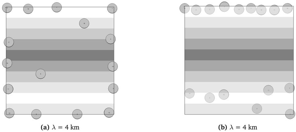
**Figure 6.25:** Wind-turbine layouts with original (left) and improved (right) OWFLO for a water depth range of 20 - 35 m, and varying wave lengths.
