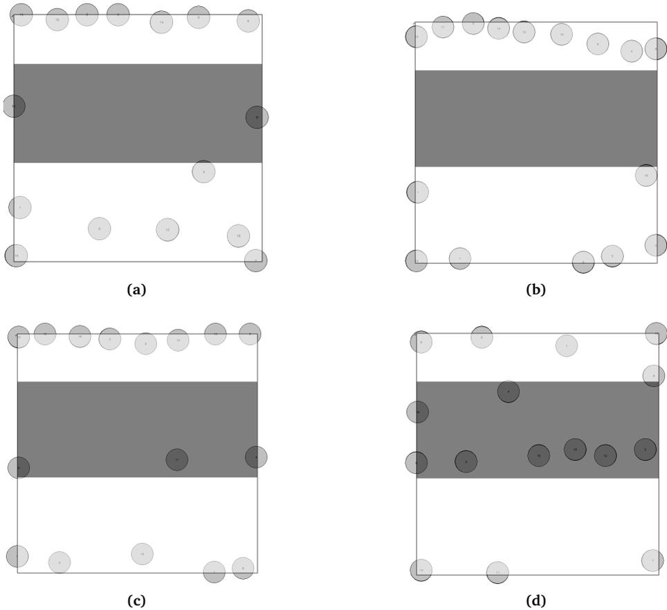
**Figure 6.10:** Wind-turbine layout for a channel width of 2000 m at 40 m water depth. Original OWFLO (a) and improved OWFLO for C50 (b), C100 (c) and C200 (d) soil type inside the glacial channel.
