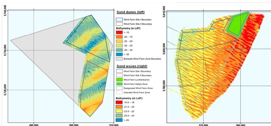
**Figure 6.2:** Sand dunes at Borssele Wind Farm Zone (left) [52]. Sand waves at Hollandse Kust Zuid Wind Farm Zone (right) [58].
