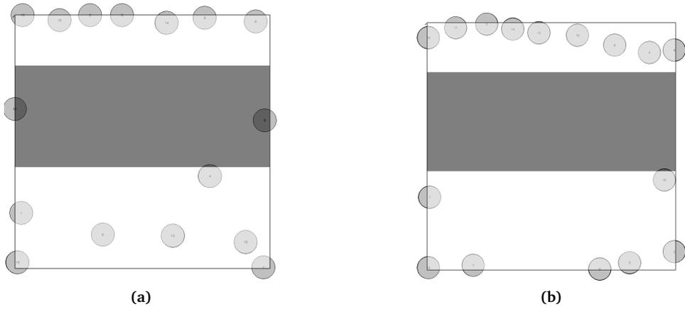
**Figure 6.17:** Wind-turbine layout for N dominated wind direction. Layouts are created with original (a) and improved (b) OWFLO.
