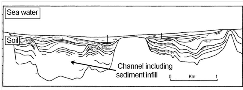
Figure 6.1: A cross section of a glacial channel in the North Sea [39].
