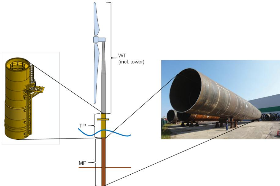
**Figure 1.1:** Impression of a WT attached to a MP foundation containing of a TP and MP [73] (c). Next to this are displayed a zoom-in of a TP including secondary steel items (l) [66] and the shell of a 7.5 m MP for Gode OWF (r) [32].
