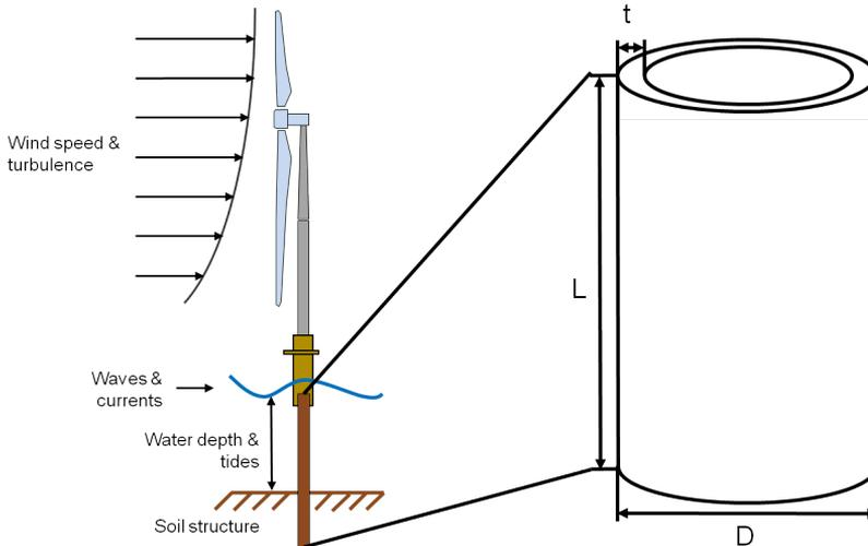
**Figure 4.2:** A visualisation of the environmental design drivers determining the geometry of the MP and therewith its mass. The drawing of the WT attached to a MP foundation is inspired by [73].
