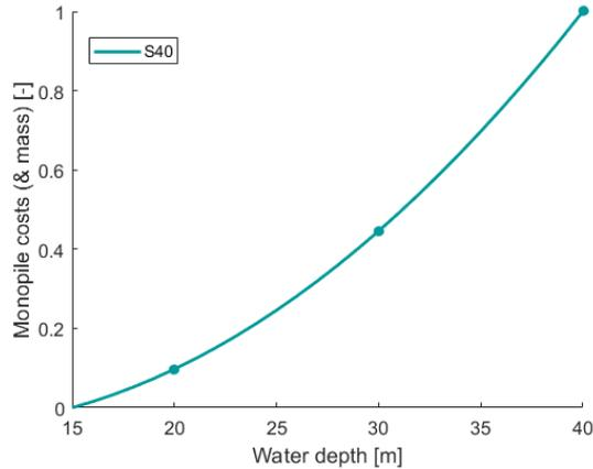
**Figure 6.6:** MP costs (& mass) against the water depth for S40 soil type. The estimations are normalized for confidentiality reasons between 0 and 1, with 0 not reflecting an absolute zero in real values. The indicators display the points for which designs are created. The plotted line is based on spline inter and extrapolation.
