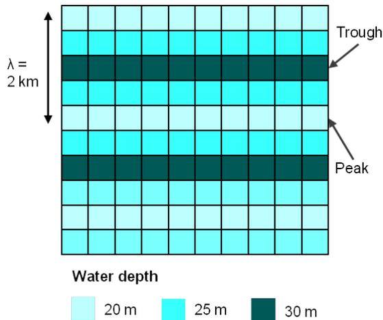
**Figure 6.4:** Visual expression of how a sand dune having a wave length of 2 km is simulated. This example has a peak to trough range of 10 m, with the trough at 20 m water depth.
