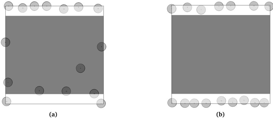
**Figure 6.14:** Wind-turbine layout with a channel width of 4000 m. Layouts are created with original (a) and improved (b) OWFLO.
