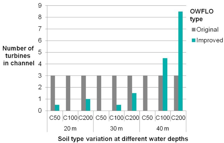
**Figure 6.9:** Comparison of the number of WTs placed inside the channel between original and improved OWFLO. This is indicated for three types of clay soil at different water depths.
