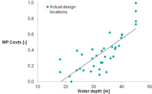
**Figure 2.4:** Scatter-plot displaying the MP costs of available designs within OWFs, plotted against the water depth. The MP costs are normalized between 0 and 1 for confidentiality reasons, with 0 not corresponding to absolute zero, but to the lowest available MP cost.
