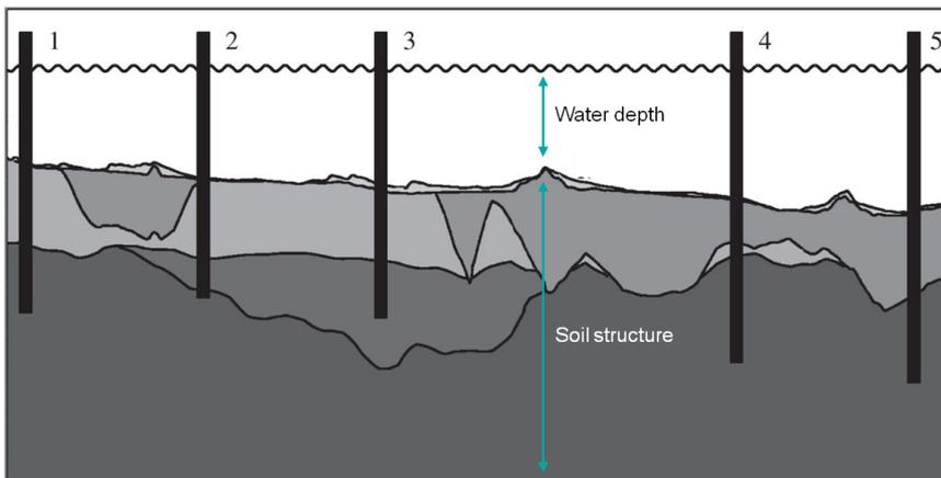
**Figure 4.3:** Cross section of soil structure and water-depth variation at Westermost Rough OWF. Indicated are MP positions (1 - 5), of which the mass reportedly varies with a maximum of 40%. The different grey colours are indicating the variation in soil structure [32].
