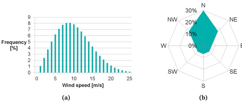
**Figure 2.1:** Distribution of wind speed (a) and direction (b) which are used in the OWFLOs of the hypothetical OWFs.
