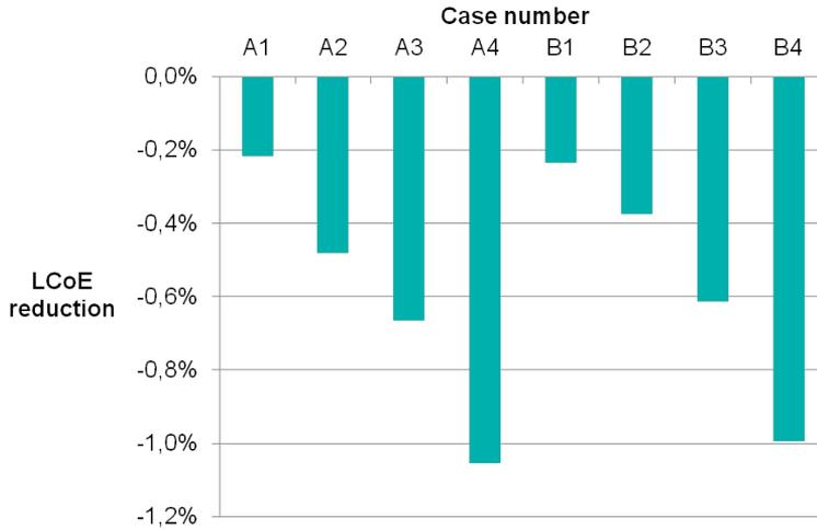
**Figure 3.2:** Percentage reduction in LCoE when MP-costs variation is included in the OWFLO process (improved OWFLO) for various MP-cost ranges and magnitudes. The case numbers are explained in Table 3.1.
