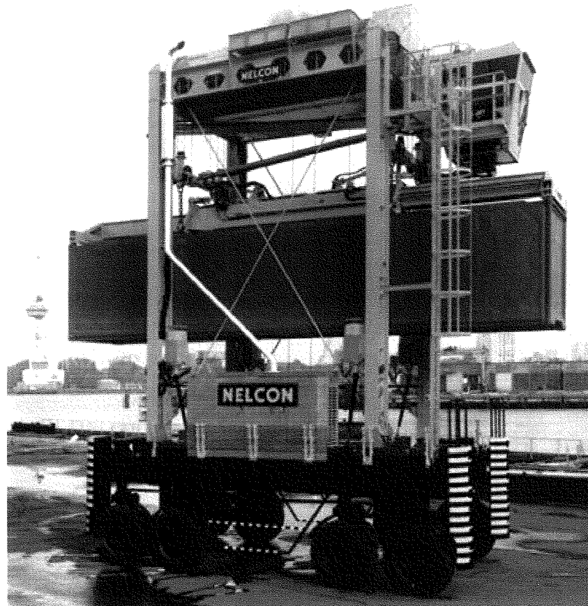
Figure 4-2 Straddle carrier, source: Nelcon
