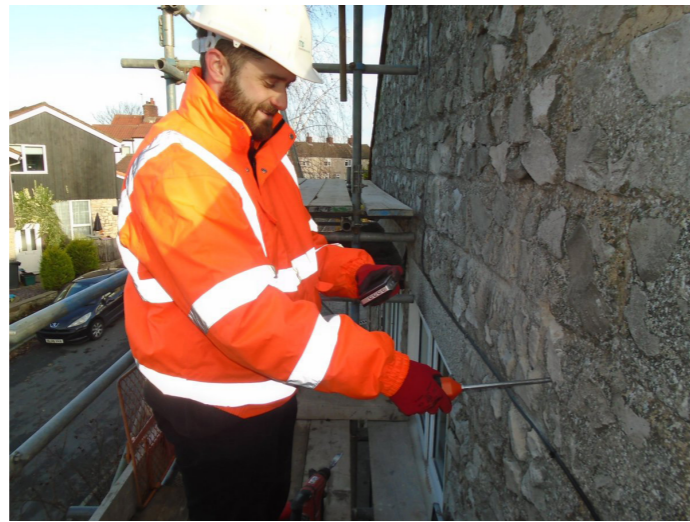
Figure 12 Endoscope in the cavity.
