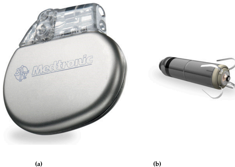
Figure 12. Modern pacemaker implanted in the chest (a) and using cables to the heart and new generation of pacemakers for complete insertion in the heart (b). © Medtronic (not the same scale).
