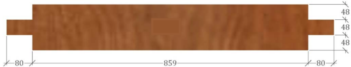
Figure 7.1: Beam dimensions [mm] of the tenon beams tested by Vermeij (obtained from [27], fig. 4.1)
