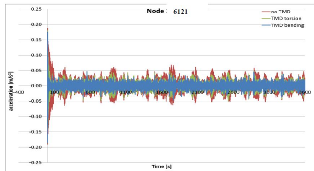
Figure 5.18: Acceleration on the top middle of the building
