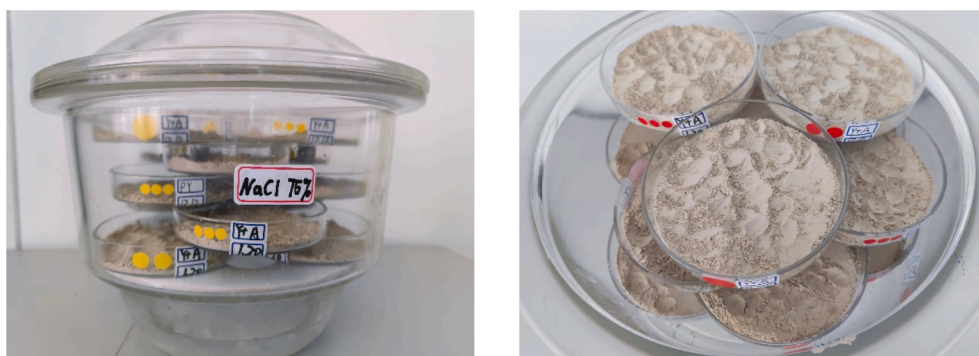
Fig. 2. The setup for cement pre-hydration.
