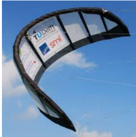
Figure 1.1: One of the LEI kites designed and used by the TU Delft AWE group for power-generation.
