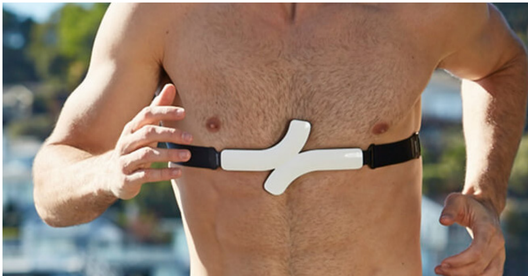
Fig 19. Qardicore body contact ecg device
