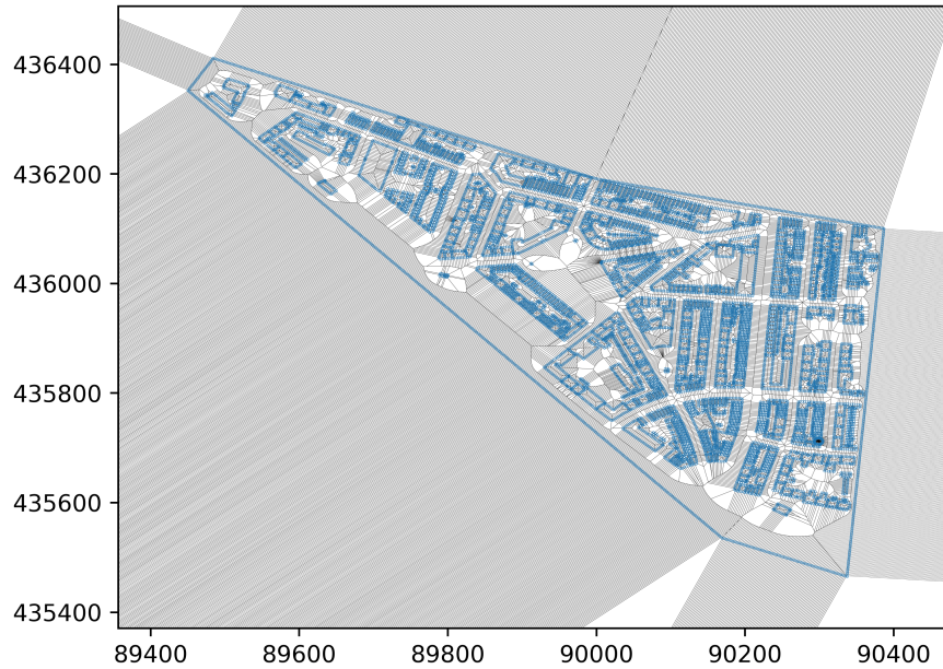
Figure 3.6: The neighborhood polygon as bounding box for creating a subset of the total Voronoi diagram
