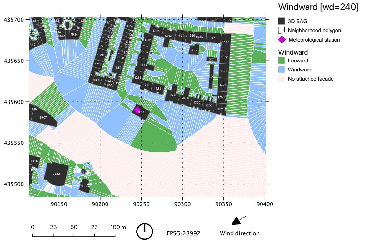
Figure 5.5: Wind- and leeward facades around the Delfshaven station for a wind direction of 240 compass degrees
