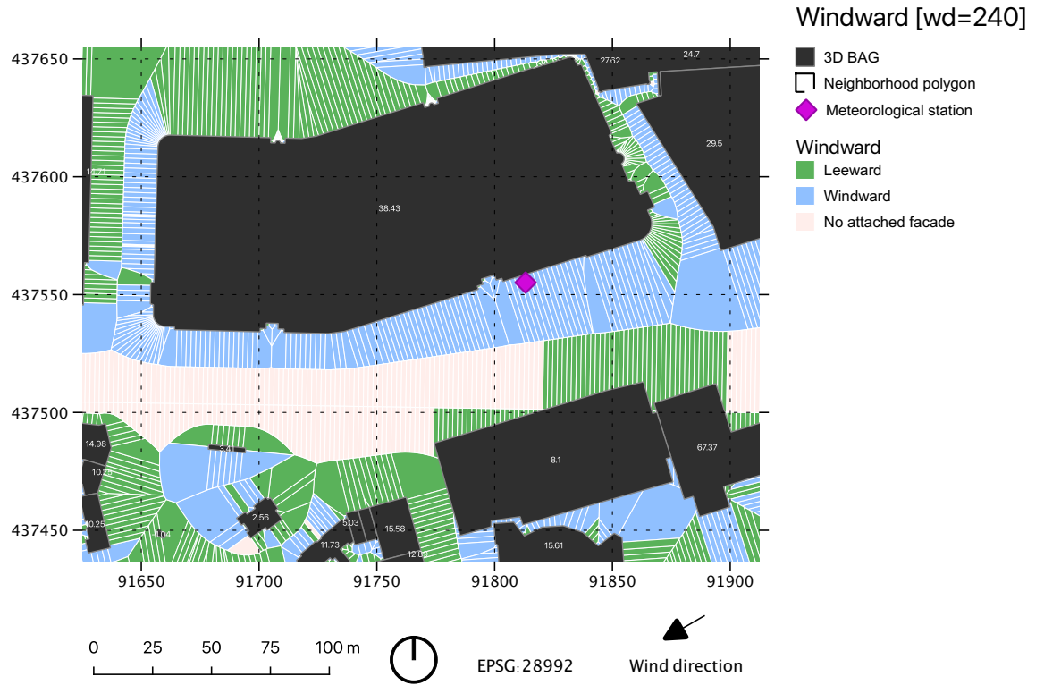
Figure 5.13: Wind- and leeward facades around the Centrum station for a wind direction of 240 compass degrees
