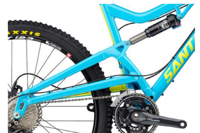
Fig. x: Santa Cruz Heckler, with a detail of the mono swingarm (Heckler, 2018)
