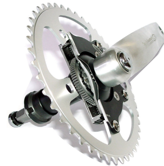
Fig. 2.35 - 2.37 top: classic derailleur, middle: gearbox - Pinion, bottom: mid gear - the Schlumpf (Wikipedia, Pinion, Schlumpf, 2018)
