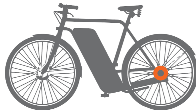
Fig. 2.30 - 2.32 top: motor in the hub of the front wheel, middle: mid motor, bottom: motor in the hub of the rear wheel (author, 2018)
