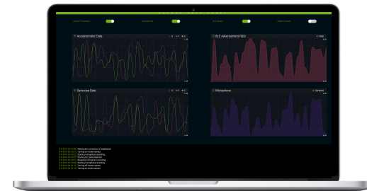
Figure 3: eSense data exploration tool showing real-time data from accelerometer, gyroscope, microphone and BLE.
