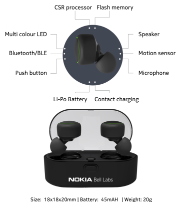
Figure 1: eSense open wearable platform with audio, motion, and proximity sensing.
