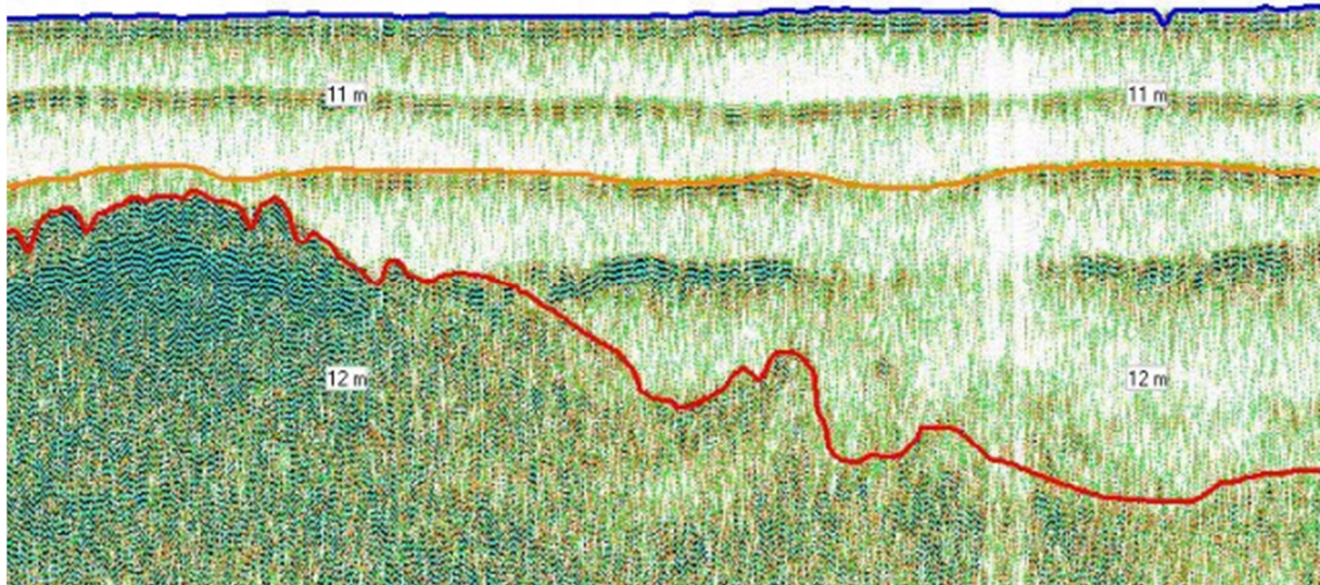
Figure 4-8 Example of analog echo sounder signal interpretation [interpretation software manual]
