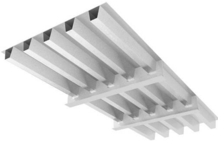
Figure 57: View of the Bottom of an Orthotropic Bridge Deck 53
