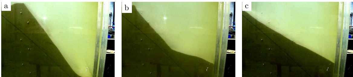
Figure 6. Initialization of a slope of 55 degrees before turning off the pump (a), 30 seconds after turning off the pump (b) and two minutes after (c).
