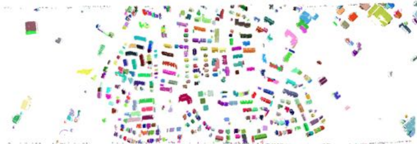
(c) Surface points corresponding to interior MAT clusters with an average separation angle of at least 70^\circ and an atom count of at least 50.
