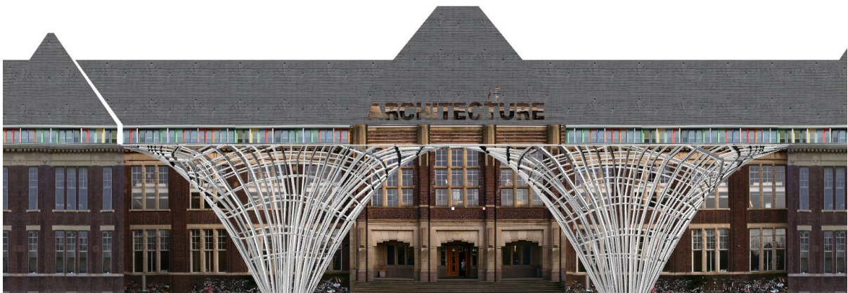
Figure 8-2: Elevation of Streamline Gridshell In Courtyard
