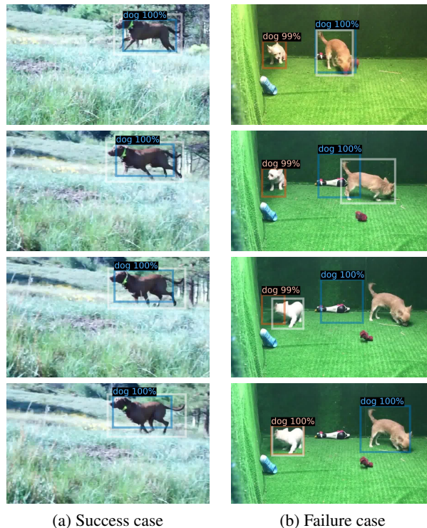
Figure 6. Example predictions. White boxes are the ground truth, blue boxes are the predictions. We show one success case in (a) a ‘dog’ running. In (b) the failure case shows a ‘dog’ suddenly changing direction. We miss the detection in the second and third frames, yet we recover at the keyframe detection. When the motion has large variations, is unpredictable, and objects enter and leave the frame, our method fails.
