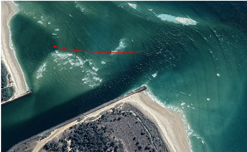
Figure 1.1: Refraction due to a channel near South West Rocks, Australia (Google, 2019). At the upper part of the channel, the waves turn away from the channel.
