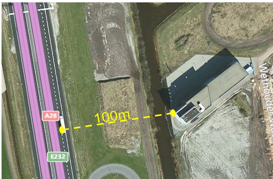
The distance from the highway is 100m, something which should be taken into consideration for choosing the appropriate LED pitch
