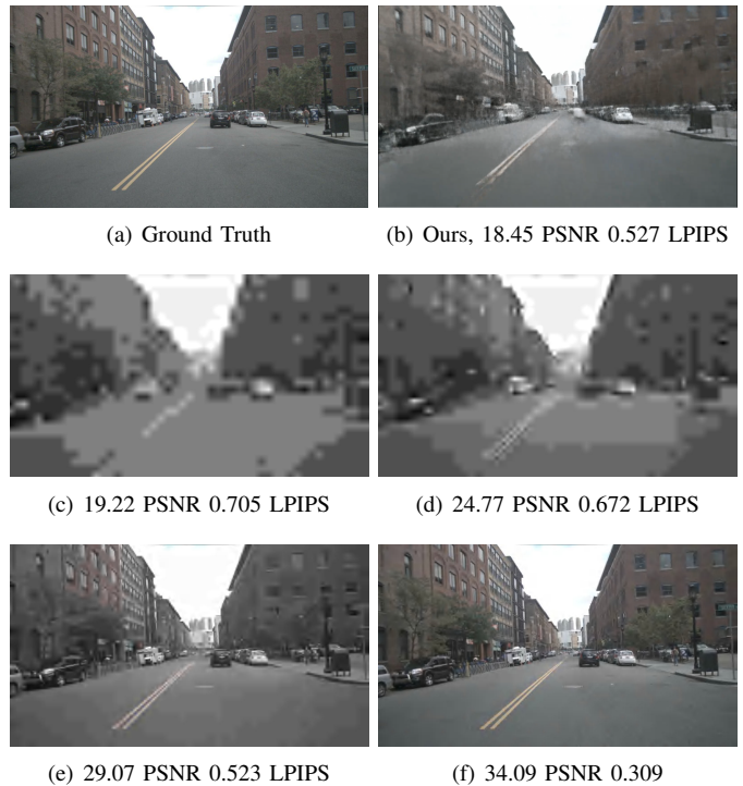
Fig. 3: A visual comparison between the JPEG2000 compressed images compressed to various PSNR (c-f) and our method (b). Here our method is able to achieve a PSNR similar to (c), though, with arguably better visual reconstruction fidelity. Specifically, our method is closer to image (e) in terms of subjective visual reconstruction performance, which has a similar LPIPS value.
