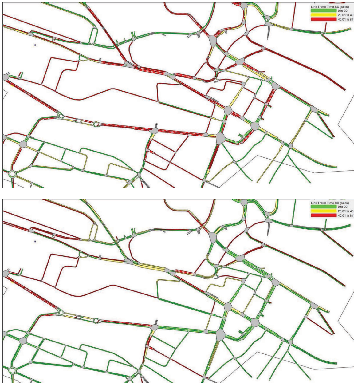
Figure 11. (Color online) Link Travel Time Standard Deviation for the Initial Plan (Top Plot) and the Plan Obtained by Solving Problem P2 with Metamodel m
