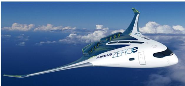
Figure 4.3: Blended wing body with aft-fuselage mounted distributed propulsion.
