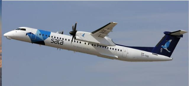
Figure 4.2: Conventional high wing design with T-tail and two wing mounted propellers.
