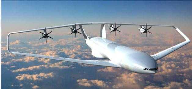
Figure 4.1: Prandtl-Box wing with aft wing mounted propellers.
