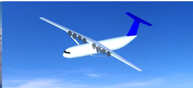
Figure 4.4: Truss-braced wing with wing mounted distributed propulsion.
