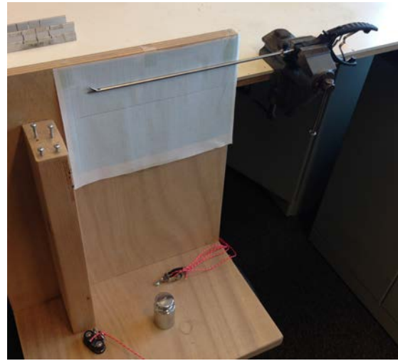
Figure 7.24: The test setup that was used to determine deflection.
