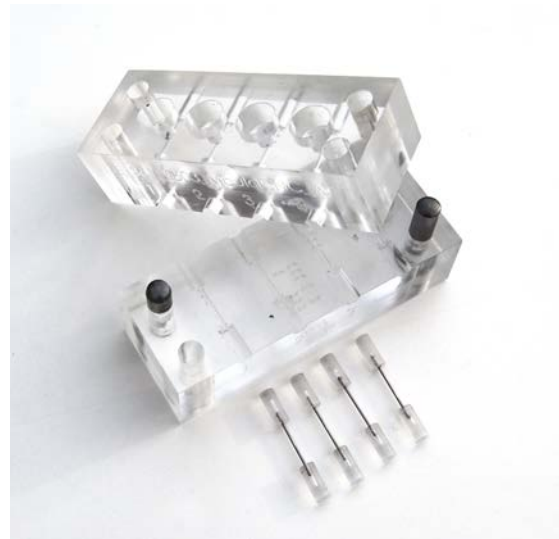
Figure 4.6: A disassembled view of the mould.
