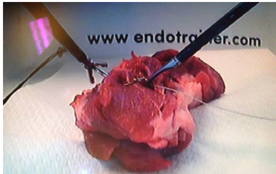
Figure 7.14: The Endohook is tested in an Endotrainer.
