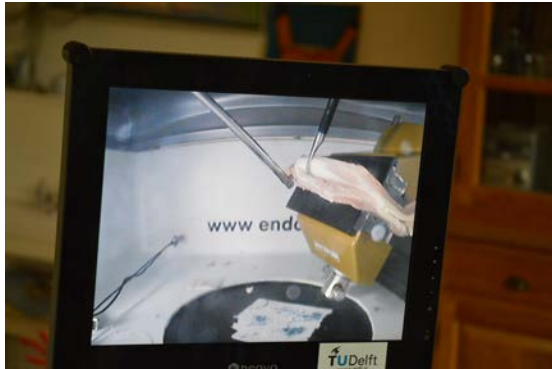
Figure 5.2: The Hornet is used in the Endotrainer to test the usability and its ability to puncture the tissue
