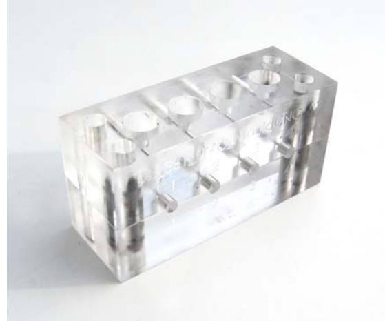
Figure 4.5: A photo of the mould that was used to cast the tacks.
