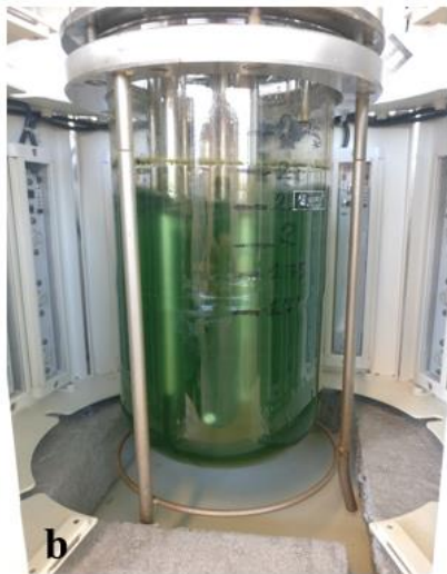
Figure 9: a. Scheme of the photobioreactor built and used for this study. Illumination was provided by a light jacket surrounding the vertical walls of the reactor. Mixing was provided by a home-made anchor paddle. In all set-ups, the temperature was kept at 35°C and argon was injected in the reactor. The incoming gas flow was controlled by a mass flow controller, while the off-gas was cooled by a condenser and passed through a cotton filter before being sent to the off-gas analyser. DO, temperature and pH were continuously measured in all set-ups. For the chemostat regime, influent and effluent flows were regulated by pumps. Acid and base were dosed in order to maintain the pH at 7. b. Picture of the reactor and the interior of the light jacket. c. Picture of the exterior of the light jacket and the interior of the PIR-boards structure. d. Picture of the exterior of the PIR-boards structure; access to the reactor was possible by an opening in the front, covered by a black plastic sheet.
