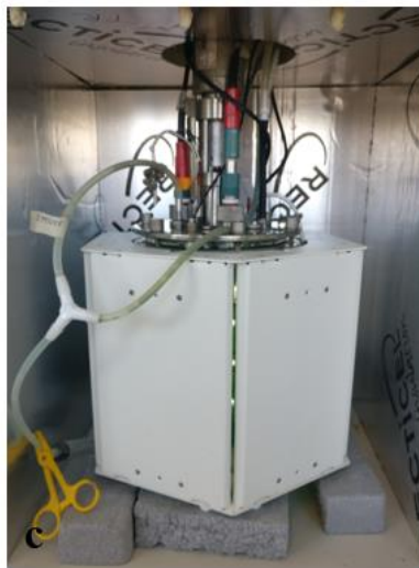
Figure 9: a. Scheme of the photobioreactor built and used for this study. Illumination was provided by a light jacket surrounding the vertical walls of the reactor. Mixing was provided by a home-made anchor paddle. In all set-ups, the temperature was kept at 35°C and argon was injected in the reactor. The incoming gas flow was controlled by a mass flow controller, while the off-gas was cooled by a condenser and passed through a cotton filter before being sent to the off-gas analyser. DO, temperature and pH were continuously measured in all set-ups. For the chemostat regime, influent and effluent flows were regulated by pumps. Acid and base were dosed in order to maintain the pH at 7. b. Picture of the reactor and the interior of the light jacket. c. Picture of the exterior of the light jacket and the interior of the PIR-boards structure. d. Picture of the exterior of the PIR-boards structure; access to the reactor was possible by an opening in the front, covered by a black plastic sheet.
