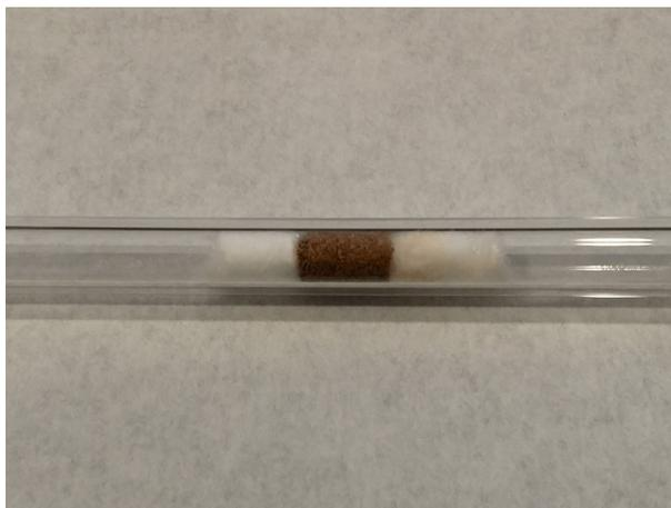
**Figure C11:** A picture of the 1Fe1Ni catalyst bed oxidized after CO<sub>2</sub> treatment (50 mg sample, 650 °C, 40 mL min<sup>-1</sup> of 10% CO<sub>2</sub> in He).
