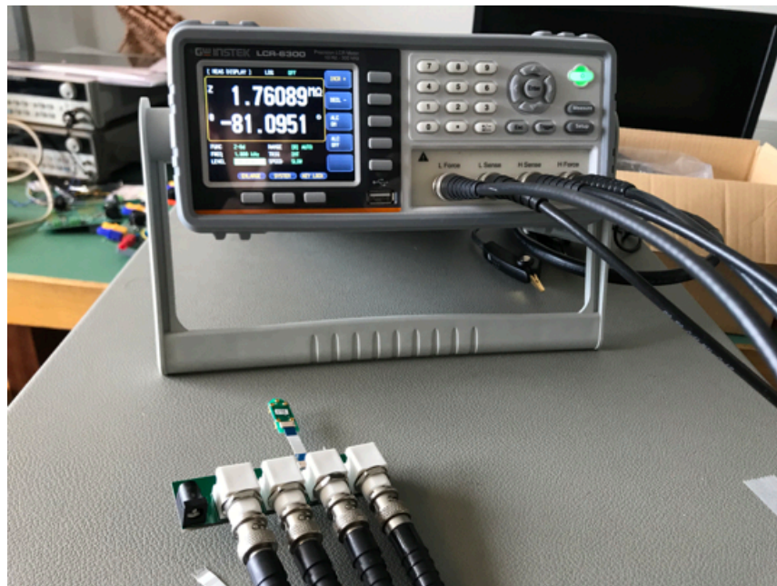
Figure 5-11 Reference measurement with LCR meter [37]
