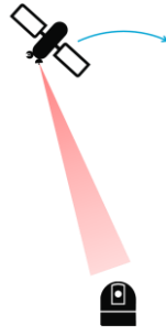
Fig. 1. Schematic view of the satellite to ground link. The satellite emits an optical beam, which contains the modulated signal. The optical ground receiver collects part of the light and relays it to the data detector. For satellites other than GEO satellites, the satellites carry speed, causing a doppler shift.
