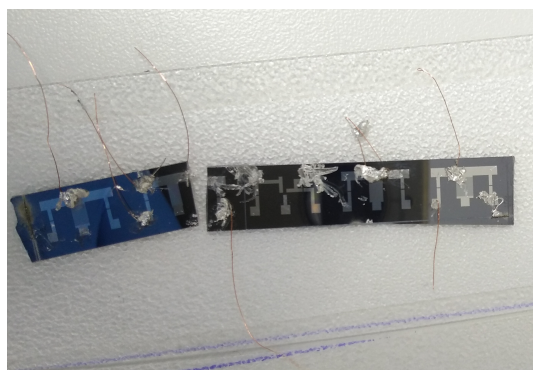
Fig. 4.8: Example of a soldered wafer sample which broke due to the points of pressure. The sample was being prepared for lamination as it fractured, and only ordinary forces were applied during handling. More information on the lamination process is provided in Section 4.2.3.
