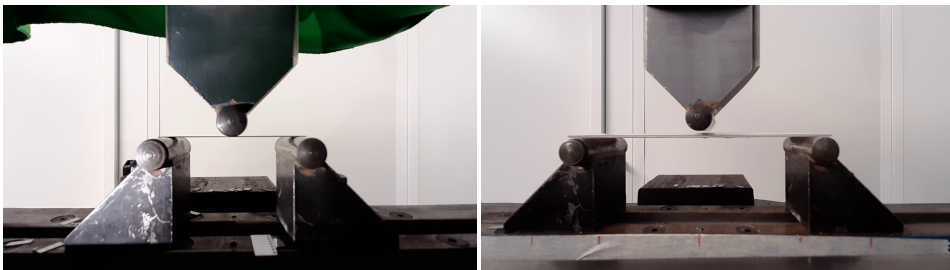
Fig. 5.13: Three-point bending test performed on bare ( left ) and laminated ( right ) wafer samples.
