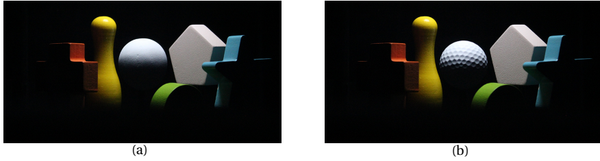
Figure 2.2: Optical mixture of scene and probe photographed from the viewing hole, with a smooth probe (left image), and a rough probe (right image).
