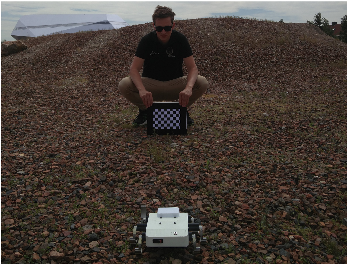
Figure 6.7: Performing Chequerboard Calibration
