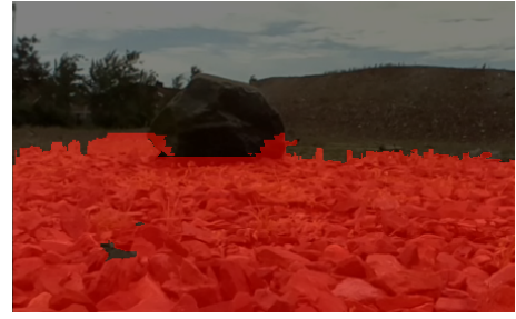
Figure 6.25: Subtracted Ground Result with Extra Hough Line Detection Step
