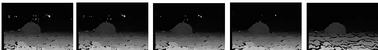
Figure 6.11: SGBM result using a block size of 5 pixels
