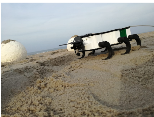
Figure 5.1: DeciZebro with external stereo camera
