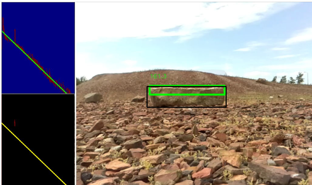
Figure 7.5: Case 1: Problem Rock seen as Ground
