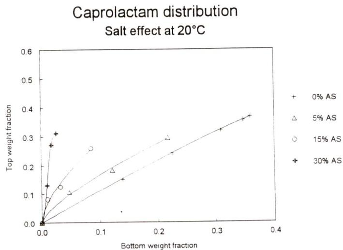
Figure 5.7: Distribution of caprolactam between aqueous (bottom) phase and organic (top) phase of the system caprolactam + water + 1-heptanol + ammonium sulfate at 20°C. Data measured by Kristina Haase. The salt concentrations in the aqueous phase were kept constant at approximately 0% w/w (+), 5% w/w (Δ), 15% w/w (○) and 30% w/w (⊕).
