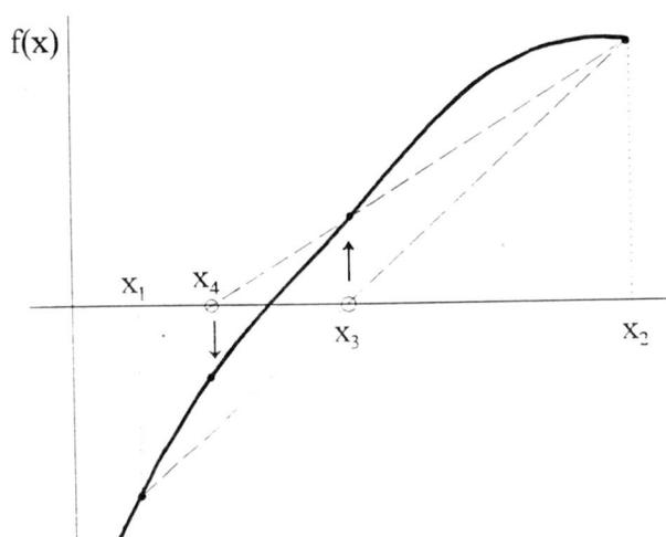
Figure 6.4: Secant method: New estimations are found by extrapolation or interpolation lines from the two most recently evaluated points. The points are numbered in the order they are used.
