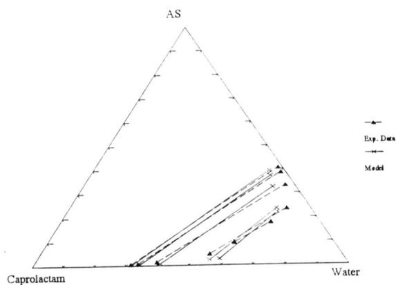
Figure 7.13: Liquid-liquid equilibrium for the system water + caprolactam + ammonium sulfate at 20°C. Representation by electrolyte NRTL + MSA. All data are in mass fractions.
