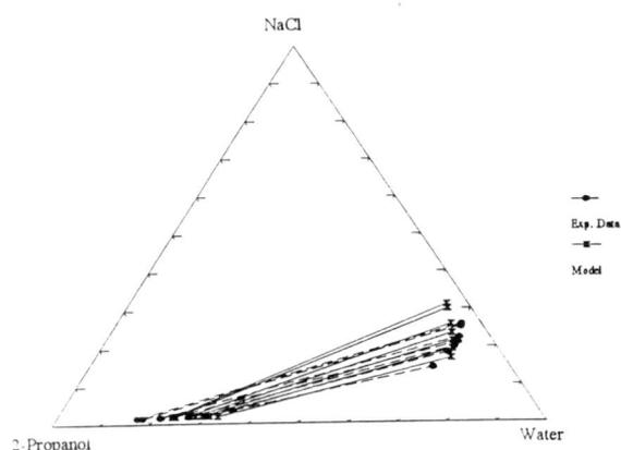
Figure 7.19: Liquid-liquid equilibrium of the system water + 2-propanol + NaCl at 25°C. Representation by the electrolyte NRTL of Chen [12]. Results obtained by Mark Wijtkamp. All data are in mass fractions.
