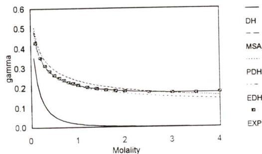
Figure 7.5: Mean ionic activity coefficients for the system water+ammonium sulfate at 25°C, calculated from the Debye-Hückel model (DH), the extended Debye-Hückel (EDH), the Pitzer-Debye-Hückel (PDH) and the MSA model. EXP = Experimental data.
