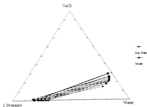
Figure 7.12: Liquid-liquid equilibrium for the system water + 2-propanol + NaCl at 25°C. Representation by electrolyte NRTL + MSA. All data are in mass fractions
