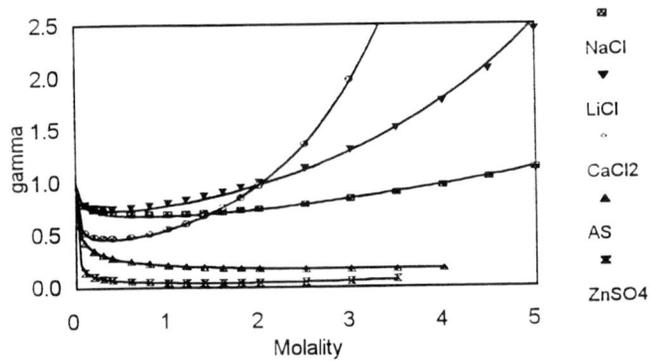
Figure 7.6: MSA mean ionic activity coefficients for salt-water systems at 25°C. Markers represent experimental mean ionic activity coefficients, lines are calculated values. Pauling diameters are used as anionic diameters. Cationic diameters were obtained by regression ( $\text{Na}^+$ : 0.325 nm,  $\text{Li}^+$ : 0.418 nm,  $\text{Ca}^{2+}$ : 0.564 nm,  $\text{Zn}^{2+}$ : 0.265 nm,  $\text{NH}_4^+$ : 0.081 nm)
