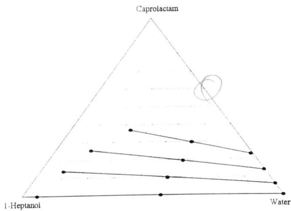
Figure 5.8: Liquid-liquid equilibrium of the system water + caprolactam + 1-heptanol + ammonium sulfate at 40°C. Data are plotted as mass fractions on a salt free basis. Solid lines represent experimental tielines, markers represent phase compositions and overall compositions. The ammonium sulfate content in the aqueous phase was approximately 5% w/w.
