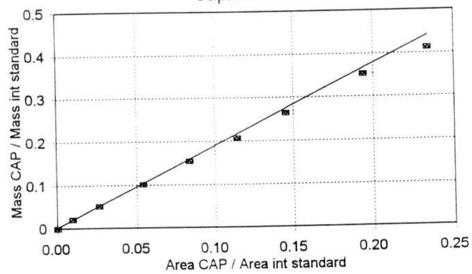
Figure I.1: Example of an regression line, used to calculate the caprolactam mass fraction of a sample with an expected mass fraction of 0.05
