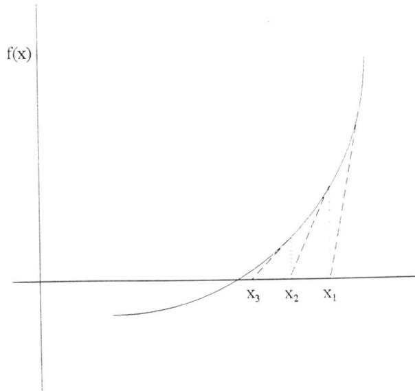
Figure 6.5: Newton-Raphson iteration: Extrapolation of the local derivatives gives the new estimation of the root. Points are numbered in the order they are used.
