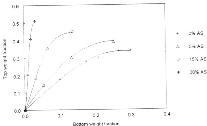
Figure 5.15: Distribution of caprolactam between aqueous (bottom) phase and organic (top) phase of the system caprolactam + water + 1-heptanol + ammonium sulfate at 60°C. The salt concentrations in the aqueous phase were kept constant at approximately 0% w/w (+), 5% w/w (Δ), 15% w/w (○) and 30% w/w (⊕)
