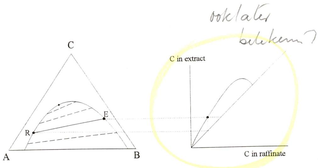
Figure 2.3: Liquid-liquid extraction is only possible when the feed solvent (A) and the extracting solvent (B) show a phase split. The streams leaving the extraction step (the raffinate R and the extract E) are in equilibrium with each other. In the figure, the liquid-liquid equilibrium is represented in a triangular diagram (left) and a distribution curve (right). [19]
