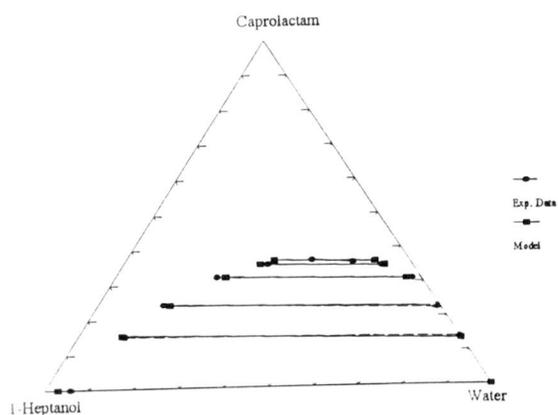
Figure 7.23: Experimental data and correlation by the NRTL model for the system water + 1-heptanol + caprolactam at 20°C
