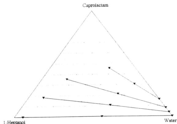
Figure 5.12: Liquid-liquid equilibrium of the system water + caprolactam + 1-heptanol + ammonium sulfate at 60°C. Data are plotted as mass fractions on a salt free basis. Solid lines represent experimental tielines, markers represent phase compositions and overall compositions. The ammonium sulfate content in the aqueous phase was approximately 15% w/w.
