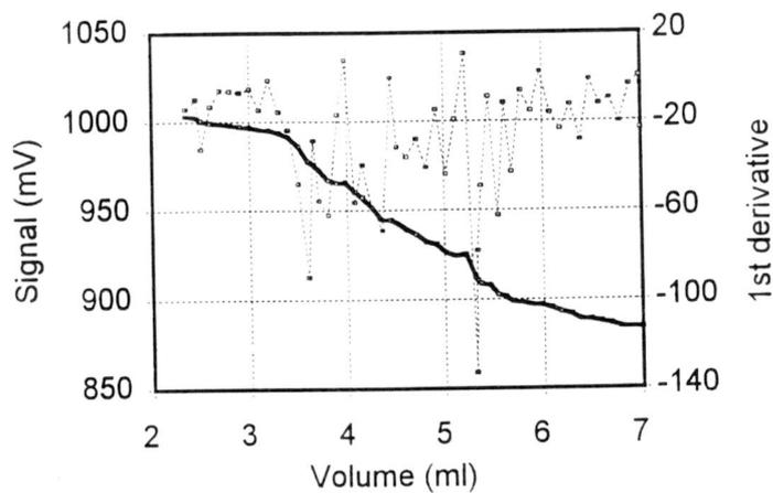
Figure V.2: Example of a result of an ammonium sulfate mass fraction determination. illustrating the difficulties of the endpoint determination.
