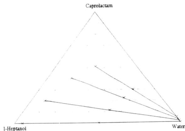
Figure 5.13: Liquid-liquid equilibrium of the system water + caprolactam + 1-heptanol + ammonium sulfate at 60°C. Data are plotted as mass fractions on a salt free basis. Solid lines represent experimental tielines, markers represent phase compositions and overall compositions. The ammonium sulfate content in the aqueous phase was approximately 30% w/w.
