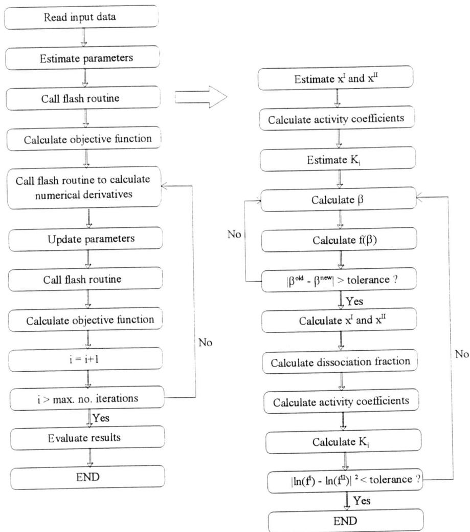
Figure 6.1: Structure of the program used to correlate experimental liquid-liquid equilibrium data of (electrolyte) solutions. Left side of the figure shows the structure of the flash routine.
