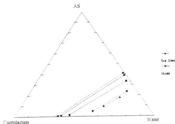
Figure 7.18: Liquid-liquid equilibrium of the system water + caprolactam + ammonium sulfate (AS) at 20°C: experimental data and correlation by the NRTL-MSA model without hard sphere contribution. The last tie-line in the critical region was not used in the regression.
