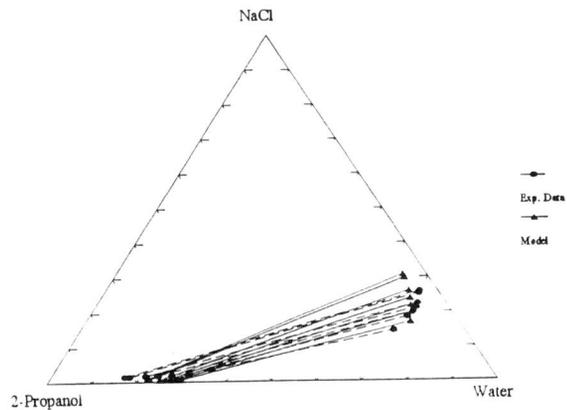
Figure 7.11: Liquid-liquid equilibrium for the system water + 2-propanol + NaCl at 25°C. Representation by the molecular NRTL combined with MSA. Dissociation constant  $K = \exp(1)$ . All data are in mass fractions
