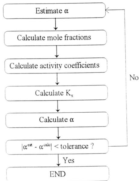
Figure 6.6: Structure of the routine to calculate the dissociation fraction.
