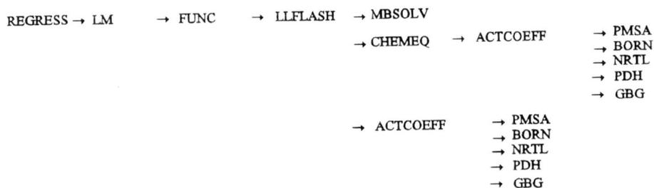
Figure 6.2: Structure of the regression part of the program used to correlate experimental liquid-liquid equilibrium data of (electrolyte) solutions. The figure contains the names of the subroutines in the FORTRAN source code. The subroutines are called from left to right and from top to bottom.
