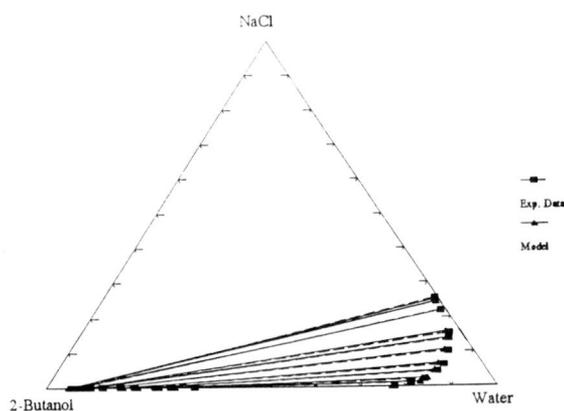
Figure 7.16: Experimental data and correlation by the NRTL-MSA model without hard sphere contribution for the system water + 2-butanol + NaCl at 25°C.
