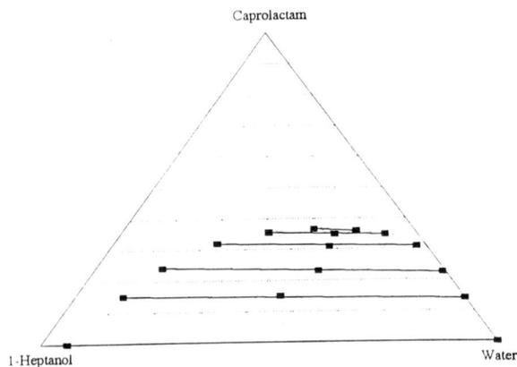
Figure 5.3: Liquid-liquid equilibrium of the system caprolactam + water + 1-heptanol at 20°C. Markers represent phase compositions and overall compositions. Solid lines represent experimental tie-lines
