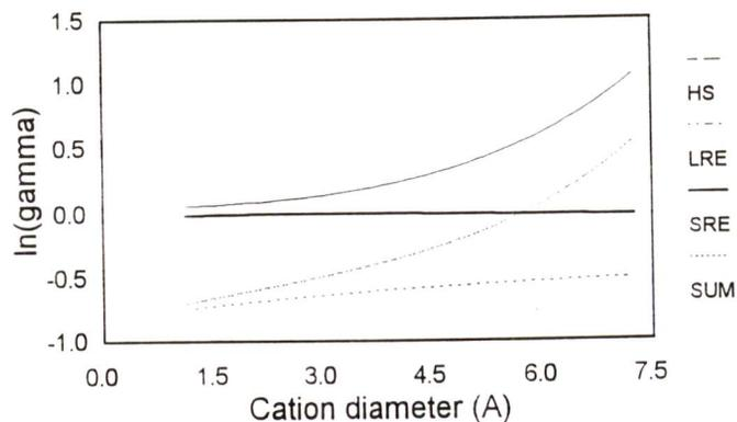
Figure 7.2: The figure shows the influence of the cationic diameter on the MSA mean ionic activity coefficient and its contributions (HS = hard sphere term, LRE = long range electrostatic term, SRE = short range electrostatic term, SUM = all contributions)
