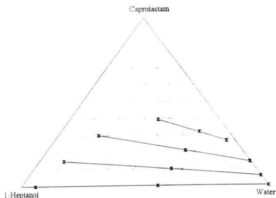
Figure 5.11: Liquid-liquid equilibrium of the system water + caprolactam + 1-heptanol + ammonium sulfate at 60°C. Data are plotted as mass fractions on a salt free basis. Solid lines represent experimental tielines, markers represent phase compositions and overall compositions. The ammonium sulfate content in the aqueous phase was approximately 5% w/w.
