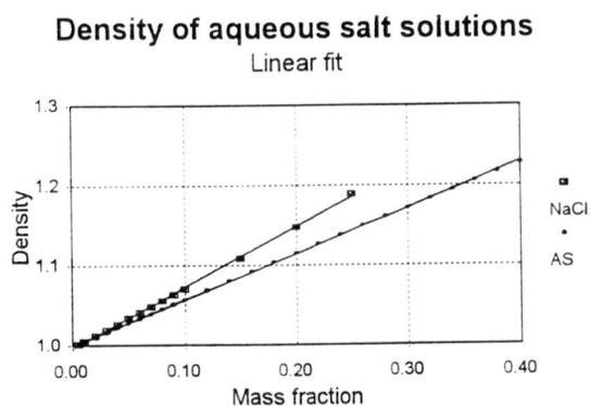
Figure 6.3: The salt effect on the density of an aqueous solution shows a linear relation with the mass fraction.
