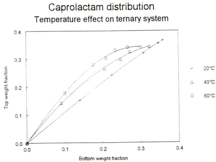
Figure 5.6: Distribution of caprolactam between aqueous (bottom) phase and organic (top) phase of the system caprolactam + water + 1-heptanol at 20, 40 and 60°C.
