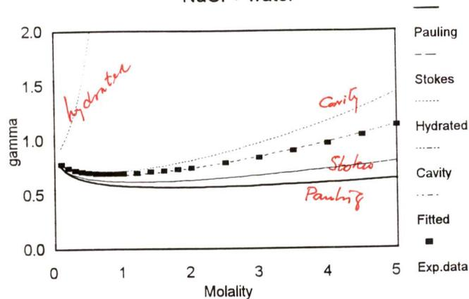
Figure 7.3: Mean ionic activity coefficient of NaCl in the system NaCl-water at 25°C, calculated with different kinds of ionic diameters
