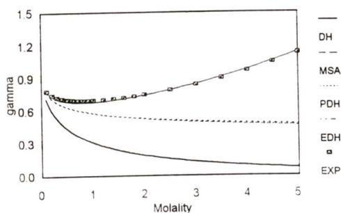
Figure 7.4: Mean ionic activity coefficients for the system water+NaCl at 25°C, calculated from the Debye-Hückel model (DH), the extended Debye-Hückel (EDH), the Pitzer-Debye-Hückel (PDH) and the MSA model. EXP = Experimental data.
