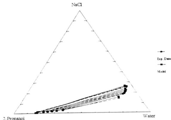
Figure 7.22: Liquid-liquid equilibrium of the system water + 2-propanol + NaCl at 25°C. Representation by the modification of the electrolyte NRTL by Liu [25],  $\alpha_{12}$  obtained by regression. All data are in mass fractions.
