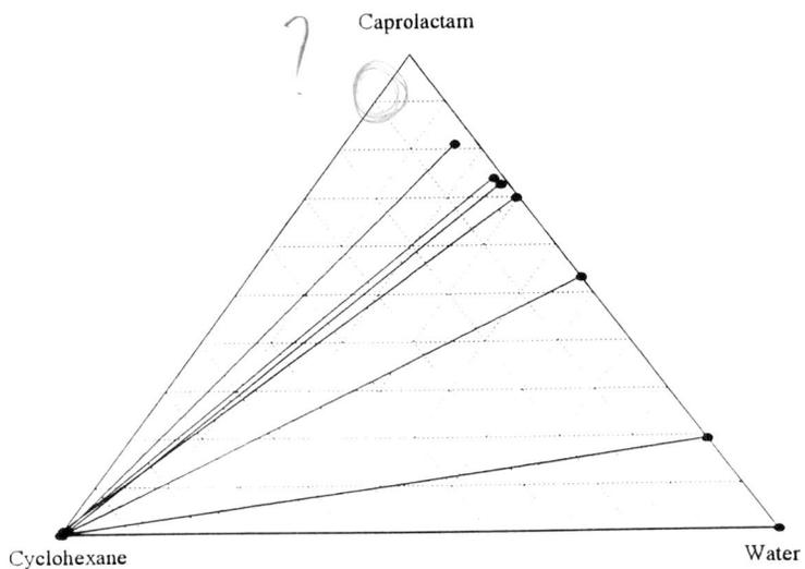
Figure 5.2: Liquid-liquid equilibrium of the system caprolactam + water + cyclohexane at 20°C. Solid lines represent experimental tie-lines. Data are plotted as mass fractions.
