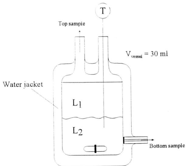
Figure 5.1: Equilibrium vessel for the measurement of liquid-liquid equilibria.
