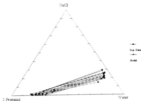
Figure 7.20: Liquid-liquid equilibrium of the system water + 2-propanol + NaCl at 25°C. Representation by the modification of the electrolyte NRTL by Liu [25]. Results obtained by Mark Wijtkamp. All data are in mass fractions.
