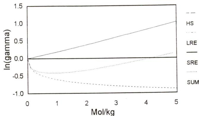
Figure 7.1: The figure shows the influence of the concentration (in mol/kg) on the MSA mean ionic activity coefficient and its contributions (HS = hard sphere term, LRE = long range electrostatic term, SRE = short range electrostatic term, SUM = all contributions)
