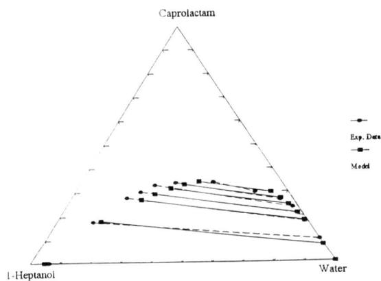
Figure 7.25: Experimental data and correlation by the NRTL model for the system water + 1-heptanol + caprolactam at 60°C
