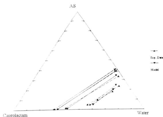
Figure 7.17: Liquid-liquid equilibrium of the system water + caprolactam + ammonium sulfate (AS) at 20°C: experimental data and correlation by the NRTL-MSA model without hard sphere contribution. All experimental tie-lines are used in the regression.
