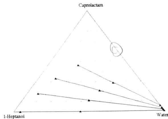
Figure 5.10: Liquid-liquid equilibrium of the system water + caprolactam + 1-heptanol + ammonium sulfate at 40°C. Data are plotted as mass fractions on a salt free basis. Solid lines represent experimental tielines, markers represent phase compositions and overall compositions. The ammonium sulfate content in the aqueous phase was approximately 30% w/w.
