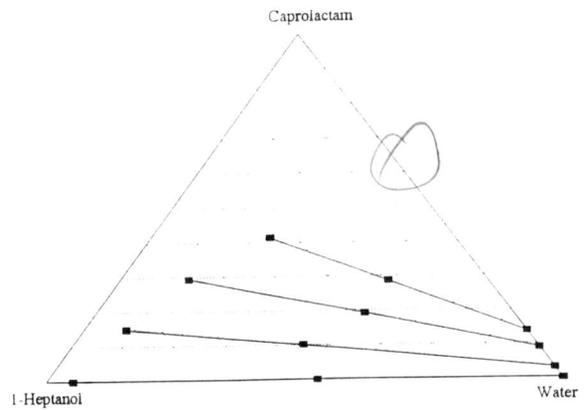
Figure 5.9: Liquid-liquid equilibrium of the system water + caprolactam + 1-heptanol + ammonium sulfate at 40°C. Data are plotted as mass fractions on a salt free basis. Solid lines represent experimental tielines, markers represent phase compositions and overall compositions. The ammonium sulfate content in the aqueous phase was approximately 15% w/w.
