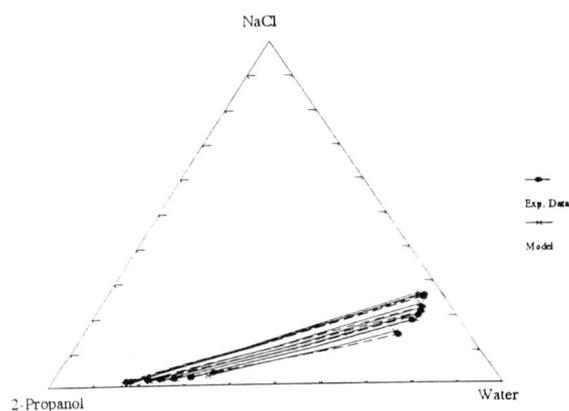
Figure 7.21: Liquid-liquid equilibrium of the system water + 2-propanol + NaCl at 25°C. Representation by the electrolyte NRTL of Chen [12],  $\alpha_{12}$  obtained by regression. All data are in mass fractions.
