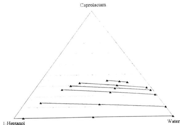
Figure 5.4: Liquid-liquid equilibrium of the system caprolactam + water + 1-heptanol at 40°C. Markers represent phase compositions and overall compositions. Solid lines represent experimental tie-lines
