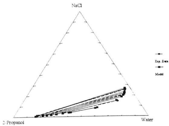
Figure 7.8: Liquid-liquid equilibrium for the system water + 2-propanol + NaCl at 25°C. Representation by the molecular NRTL. All data are in mass fractions.
