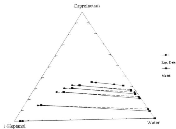
Figure 7.24: Experimental data and correlation by the NRTL model for the system water + 1-heptanol + caprolactam at 40°C
