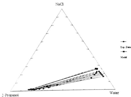
Figure 7.10: Liquid-liquid equilibrium for the system water + 2-propanol + NaCl at 25°C. Representation by molecular NRTL combined with MSA. All data are in mass fractions.
