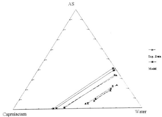
Figure 7.9: Liquid-liquid equilibrium for the system water + caprolactam + ammonium sulfate at 20°C. Representation by the molecular NRTL. All data are in mass fractions
