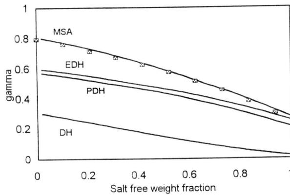
Figure 7.7: Mean ionic activity coefficients for the system water + methanol + 1 mol/kg LiCl at salt free methanol fractions of 0 to 1 kg/kg. Markers are experimental values, lines represent calculated values. (MSA = Mean Spherical Approximation, EDH = Extended Debye-Hückel, PDH = Pitzer-Debye-Hückel, DH = Debye-Hückel)
