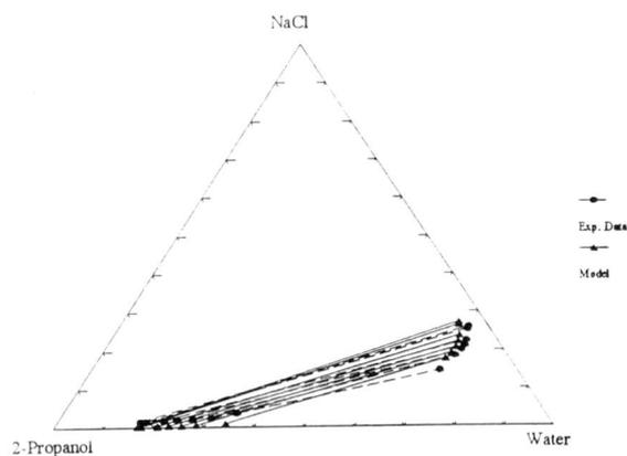
Figure 7.14: Liquid-liquid equilibrium of the system water + 2-propanol + NaCl at 25°C. Representation by the electrolyte NRTL + MSA (without hard sphere contribution). All data are in mass fractions.
