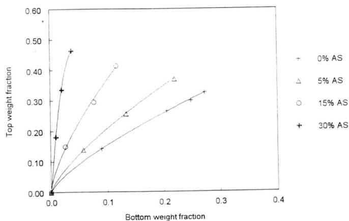
Figure 5.14: Distribution of caprolactam between aqueous (bottom) phase and organic (top) phase of the system caprolactam + water + 1-heptanol + ammonium sulfate at 20°C. The salt concentrations in the aqueous phase were kept constant at approximately 0% w/w (+), 5% w/w (Δ), 15% w/w (○) and 30% w/w (⊕)
