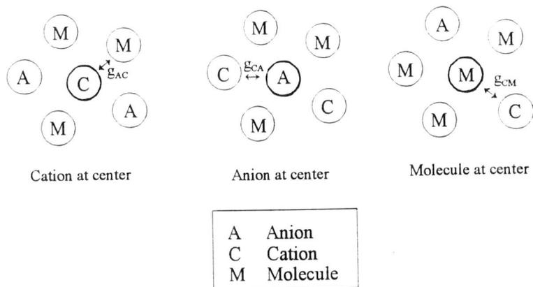
Figure 3.1: Three types of cells in the electrolyte NRTL, according to the like-ion repulsion and local electroneutrality assumptions. [13]
