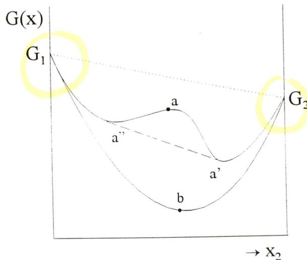
Figure 2.4: Gibbs energies of binary mixtures as functions of composition. The portion a'-a-a'' of the upper curve represents an unstable region. In this region the lowest Gibbs energy is reached by splitting into two phases with compositions a' and a''. The lower curve is that of a completely miscible mixture.[48]
