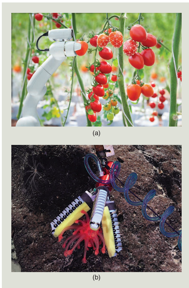
Figure 5. Two examples of interactions with fragile objects that could benefit from the use of soft robots. (a) Picking tomatoes [19]. (b) A custom 3D-printed soft robotic gripper, grasping mushroom coral [20].
