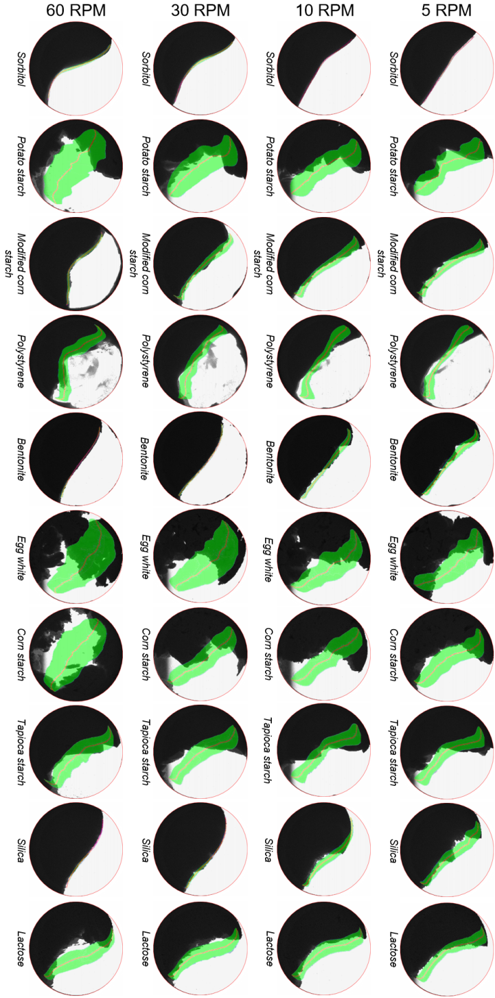
Figure 6.6: Representative snapshots of the flow pattern of the powders at rotation speeds of 5, 10, 30, and 60 RPM, ordered from top to bottom. The mean (red line) and standard deviation (green area) of the powder surface position are superimposed with transparency over the flow pattern images. Video S1 displaying the flow behavior is included in the electronic supplementary of the article.
