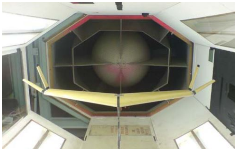
Figure 1.4: Picture of the model with articulated split wingtips used in the wind tunnel tests [8]
