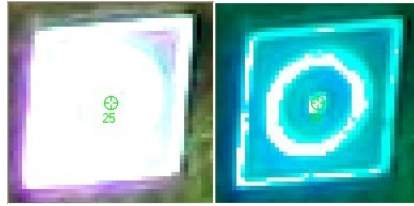
Figure 7.4: GCP blinded by sunlight (left) and result of histogram adaptation (right)
