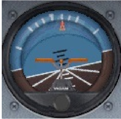
Figure 6.2: Standard artificial horizon used in full sized aircraft, as represented in Microsoft Flight Simulator X
