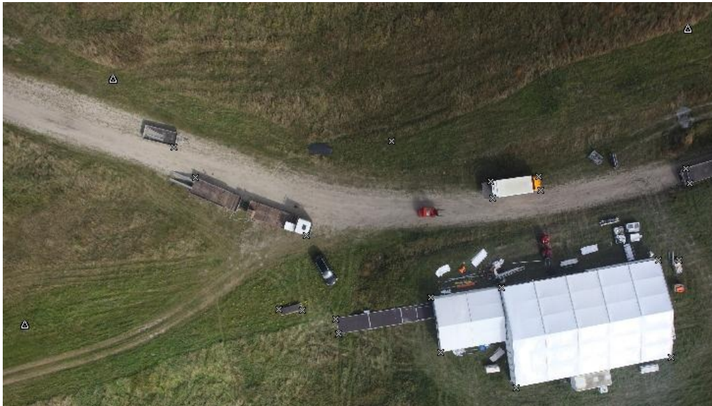
Figure 6.3: Example of GCP and tiepoint collection in PhotoModeler, the small triangles are GCP's marked in Photomodeler, the small crosses are extra tiepoints.
