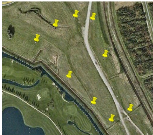
Figure 6.1: Test area with Ground Control Points as tags, image taken from Google Earth
