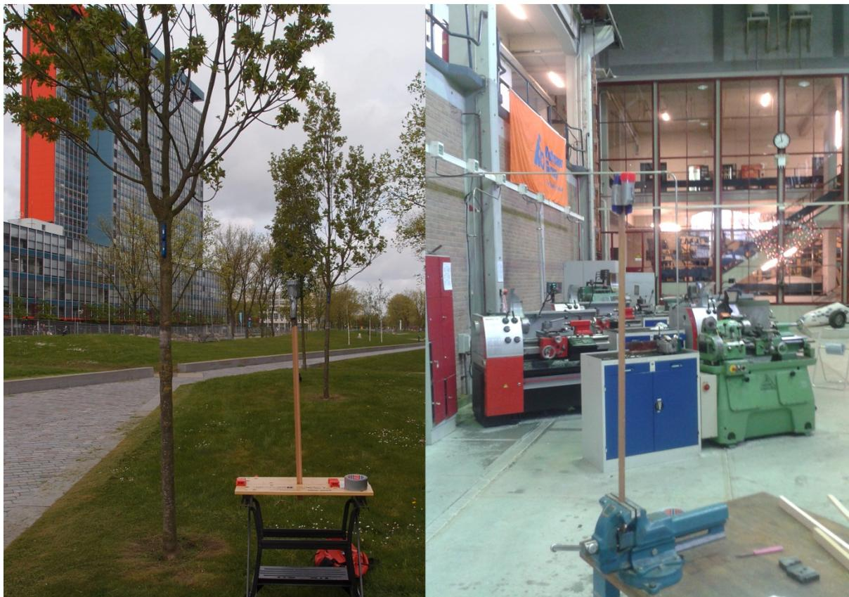
Figure 5: Left: The set up for the wind experiments on a stick and a tree, right: sway experiment setup.
