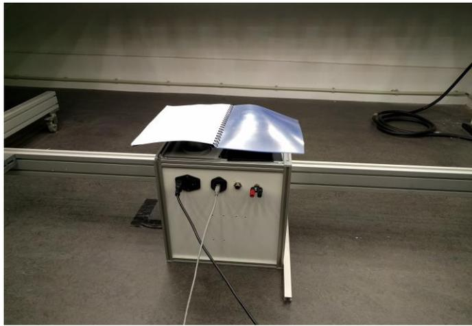
**Figure 18: With the plastic screens for shading testing under the LASS.**
