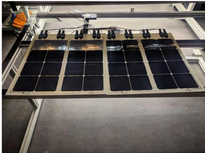
Figure 41: The 4 x 4 Wiring Configuration with two panels in series.
