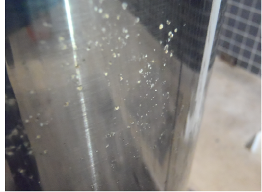
Fotonr. 24: indicaties in cilinderstang – detail 1
