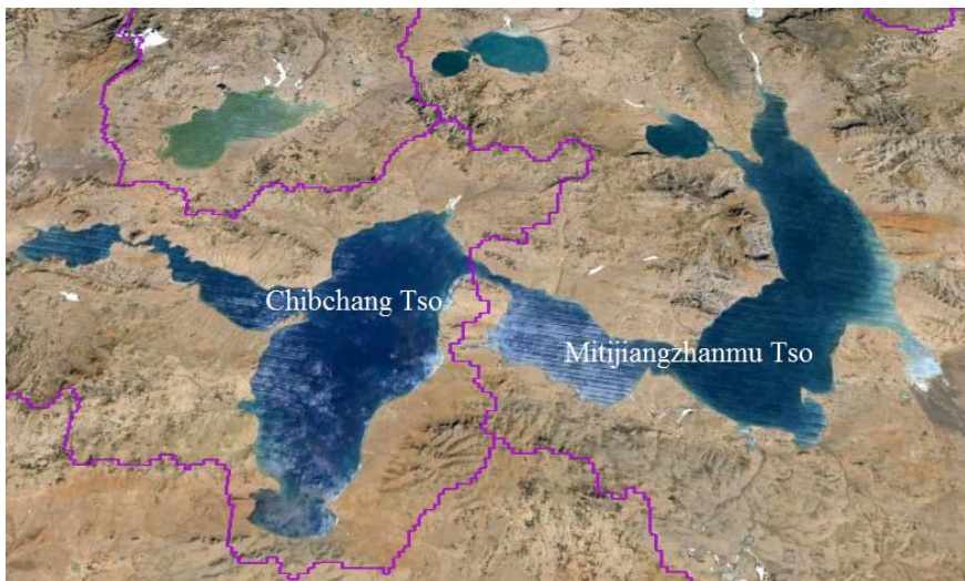
Figure 6.12: Effect of the low resolution of SRTM in the separation of Chibchang Tso and Mitijiangzhanmu Tso into two closed catchments derived from the HydroSHEDS drainage basins when overlaid on Google Earth.
